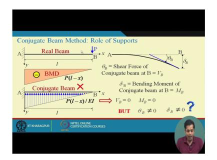
Now why it cannot be the conjugate beam? Because one aspect of conjugate beam is the loading. That loading on the conjugate beam is M by EI diagram of the real beam and another aspect of the conjugate beam is the support condition. Is it that whatever support we have in the real beam, is it the same support the conjugate beam also have or the conjugate beam has different kinds of support? Okay. So now next you will see that in order to form a conjugate beam, two steps are required.
