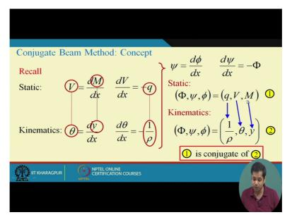
So the problem is reduced to determine determination of shear force and bending moment of the conjugate beam. And once we do that directly shear force and bending moment will give us the other kinematic variables of the real system. And this is the concept behind conjugate beam method. We demonstrated one small example where a simply supported beam subjected to uniformly distributed load. Now so that was the problem we discussed in the last class.
