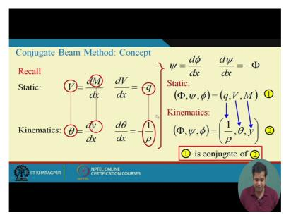
Before we go further let us once again review this. The idea has been, we have two problems. One is the problem of statics, one is a problem of kinematics. Problem of statics tells you that we have a structure subjected to some external load then the static problem is determine the internal forces in the structure and the static equilibrium is the premise of that process.
