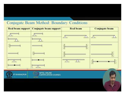
And similarly if the real beam is an internal hinge, what is the internal hinge in the real beam? In real hinge rotation is possible but in this case now rotation is possible means what? Rotation corresponds to shear force. So your beam will be such that shear force is non zero.
