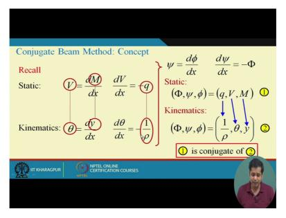
Now we discussed in the last class that the q curvature is conjugate to q or deflection is conjugate to M or theta is conjugate to V. Now you have real system where we need to find out the curvature, slope and deflection and then what we have to do is we have to construct a conjugate system where the intensity of the load is replaced by the curvature of the real system means M by EI diagram of the real system.
