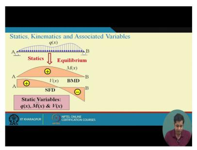
So in this entire step our static variables are intensity of the load, bending moment and shear force, right? Now this is not the only thing we want. What we want in addition to internal forces are deflection of the beam. Suppose this beam deflects like this, okay.
