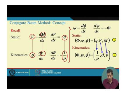
Now in this case it is called that system 1 is conjugate of system 2. So how this conjugate is obtained? Conjugate is obtained by replacing q by curvature of system 2. So only thing we have to do is in order to get the conjugate system 1 we have a system 2. Now in order to get the conjugate system 1 we have to replace the intensity of intensity q by 1 by (ra) rho in the curvature of system 2. Now if we do that then what you have to do?
