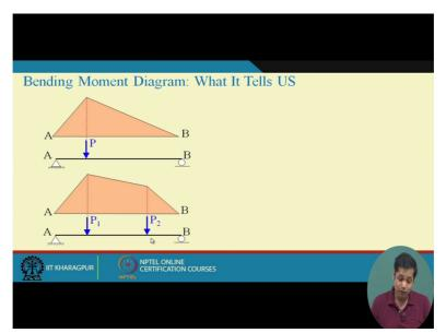
And not only that, after reaching this point bending moment decreases, this value is lesser than this value. We can also say that P1 should be greater than P2 or P2 should be less than P1.
