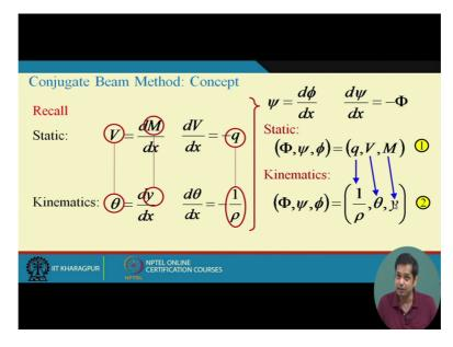
Now since in system 1 suppose if q is replaced by curvature, okay, if q becomes curvature then curvature of system 2 then (natu) automatically the shear force of system 1 becomes slope of system 2 and the bending moment of system 1 becomes deflection of system 2.
