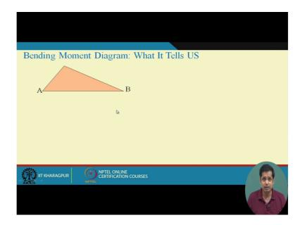
Now what this bending moment diagram tells you? That suppose it is also known that we have a support at A and support B. Now bending moment is zero at support A and bending moment is zero at support B. So the support condition on the real beam will be there will be no constraint against rotation. So naturally it will be hinge support and it will be roller support or this is hinge support, this is a roller support, okay.
