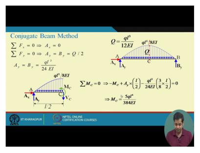
Now what we have? Shear at A is equal to the support reaction at A which is equal to qL cube by 24 EI that we already obtained what is the support reaction. What will be the shear at B? Shear at B will be minus By not AB, okay.
