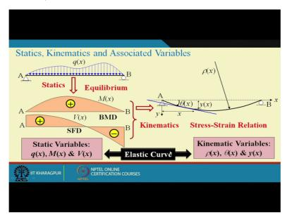
And if you observe from the last week whatever method we studied in determination of deflection of beams, the premise of all the method is elastic curve. They use the equation of
