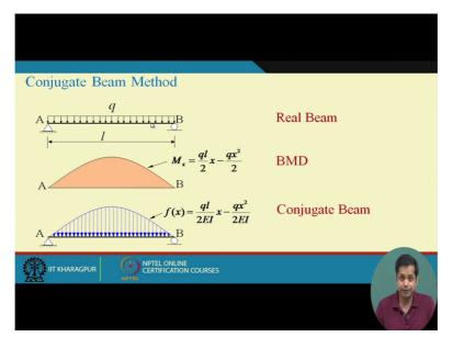
Now this is conjugate beam method. Now this is the conjugate beam where in real beam it was uniformly distributed load. Now in conjugate beam the load is replaced by the bending moment by EI. This was the bending moment M by EI. How the M by EI changes with the x and we also know that the maximum moment is qL square by 8. So this point becomes qL square by 8 EI.
