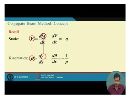
Now how V is related to q and how theta is related to curvature that is also very similar. So what we can say the shear force is the first derivative of moment and here theta is first derivative of deflection. First derivative of shear force is intensity of the loading, first derivative of slope is equal to the curvature.
