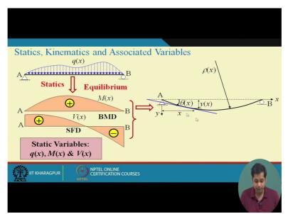
So these are the two responses we want from structural analysis. Now from this step once we know the internal forces on a structure and from that internal forces (app) determine the deflection. This step is called kinematics. Kinematics essentially is the branch where we determine the motion of an object as a relation with the forces that causes the motion. In this case motion is the deformation or deflection of the beam, okay. So this step is called kinematics.
