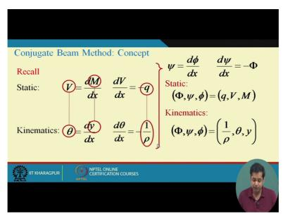
So this is the general equation which gives you static and kinematic equation depending on what psi, phi and capital Phi are chosen. Now what point I want to make here? You see if q is replaced by 1 by rho then V, the shear force will be replaced by theta and similarly moment will be replaced by y.
