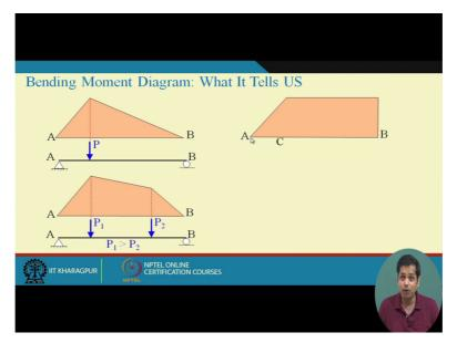
Since we have a (pos) non zero bending moment here means either we have externally applied moment or the support is fixed support. So this could be the beam and the loading condition could be like this because this is constant. So since this is constant so this is the loading condition we will have.
