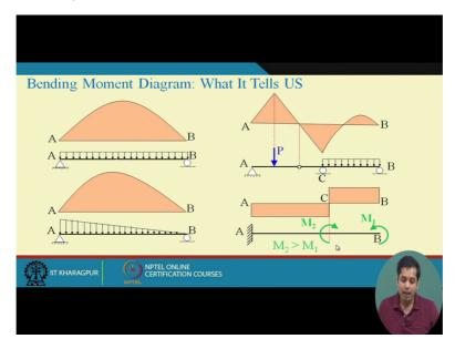
Now so if we have bending moment diagram and that is true for shear force diagram as well. If we have bending moment diagram and shear force diagram then we can get some information from those diagrams. We can have some idea about the support conditions of the structure and the loading conditions of the structure. Now but whether these loading conditions are unique or not that I leave it to you. That would be for all the bending moment I (sho) showed here.
