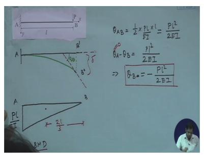
Now since A slope is zero, so this projection itself gives you the deflection at point B. So what will be the deflection at point B? So Yb, or you can write delta B as well. Delta B is equal to moment of this M by EI diagram about point B. So this area is PL square by 2EI. PL
