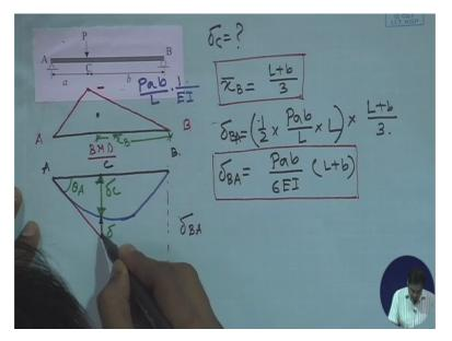
Now, then what is delta? Delta is essentially the deviation of point C.On deflected shape this is point C. So it is, delta is equal to deviation of point C with respect to slope at A. So it is essentially delta CA, right?
