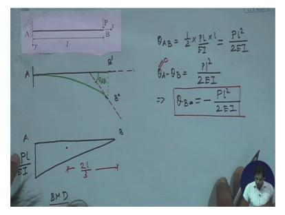
Now what will be the deflection? Now moment area method doesn't tells you directly about the deflection. What it tells you? That the deviation of or the projection of any point on a slope drawn at another pointwill be the moment of the M by EI diagram about the concerned point at which the deflection needs to be measured. So in thiscase what we need to do is. This is delta, right? This is the projection of B onto the slope drawn at A.
