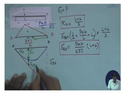
Now again applying moment area method and what would be delta CA? Delta CA will be the moment of M by EI diagram between A and C aboutfrom C. So the delta CA will be moment of this diagram. Moment of the bending moment diagram between A and C is this, this triangular portion. Moment of this diagram about point C here.
