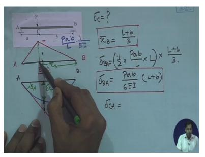
So this will be then, half Pab by EIL. Here also it should be EI.And into A. This distance is A, into A by 3. The centroid of this triangular area from point C is A by 3. So this becomes Pa cube b divided by 6EIL, delta CA. So delta CA is not the deflection at C. Delta CA is the deviation of point C with respect to slope drawn at point A. And remember one thing, when we are talking the deviation, it is the deviation is measured from the deflected shape of the
