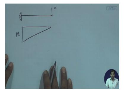
And similarly we can draw bending moment diagram for any problem. Now this bending moment diagram depends only on what? Only on this applied load. For given length of the beam, this bending moment depends on the applied load. If P is more, then bending moment is more. If P is less, then bending moment is less. It does not depend on what material the beam is made? What would be the cross section of the beam? Right?
