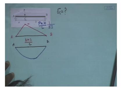
Now so first draw a slope at point A. So this is slope at point A. Now, so this is theta A, right? Now if this is point B, then projection of point B on the slope drawn at A, this point is B dash. And this distance is delta BA. So this means that this is deviation of B with respect to the slope drawn at A. So this is delta BA, right?
