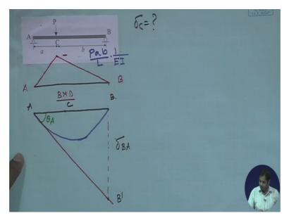
Now momentarea method says that this deviations delta BA will be the moment of the M by EI diagram about this point B. Now moment of this diagram will be, area of this diagram multiplied by the centroid distance of the diagram from B. Now you can verify yourself that if this is a centroid of this entire triangular area and this distance is XBof that. XB bar, that's what we use.
