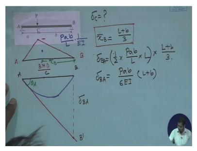
So we have obtained the deviation of B with respect to the slope at A, delta BA. What is the question? Question is we need to determine this distance. If this is delta C, we have to determine this distance.
