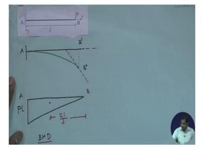
So as per moment area method we know that theta AB which is the angle between the slopes drawn at A and B. So slopes drawn at A is this and slope drawn at B is this. So angle between this angle is theta AB, right? And we know that theta AB will be the area of bending moment diagram between A and B. So area of bending moment diagram means this.
