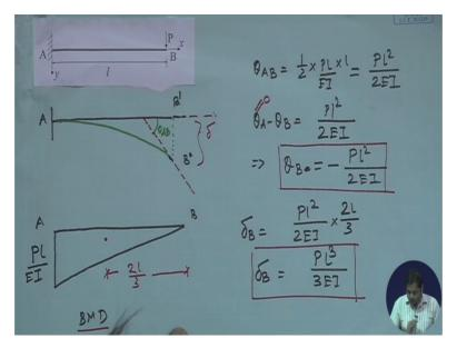
So this is again a very standard result. A cantilever beam subjected to tip load. The deflection at the free end is PL cube by 3EI. So this is again a very simple problem. Now you verify this results with the results that you obtained usingdirect integration method. Now let's see one more example. This example is a simply supported beam subjected to concentrated load at any arbitrary point between A and B.
