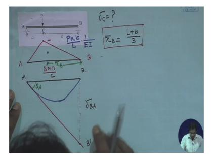
So what would be deviation delta BA? Delta BA will be the area multiplied by this distance. So delta BAwill be, the area of this diagram is half into Pab by L into L. This is the total area multiplied by this distance XB which is L plus B by 3. So this becomes Pabby 6EI into L plus B, delta BA.
