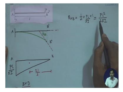
Now what is angle between A and B? Theta A minus theta B, right? Theta A minus theta B is equal to PL square by 2EI. Now slope at A is equal to zero because it is fixed end. So this is equal to zero. So this gives us theta B is equal to minus PL square by 2EI. So this is slope at free end. Theta AB is equal to theta B minus theta B. So this is the slope.
