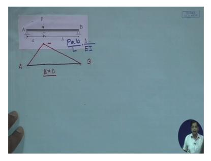
In this case please note EI is constant. That's why we can directly divide bending moment by EI. So this distance is this distance. Now first draw the deflected shape of the beam. So this was the original configuration of the beam and the deflected shape of the beam will be something like this.
