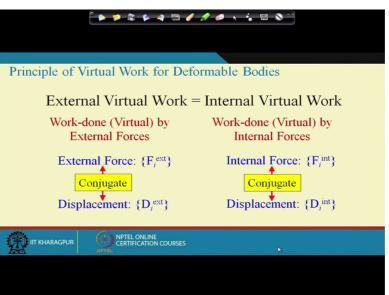
Now before we actually go further in deriving the expression of the principle of virtual work let us understand what we (un) mean by external. There are four parameters involved here, okay. External forces, internal forces and the external displacement and the internal displacement. Let us now understand and these four ingredients they constitute the principle of virtual work for deformable bodies.
