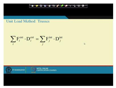
Now what is the external load we have? External load we have in the system 1 is this. That is the external load, okay. The points B does not move so there is no work done by the reaction
