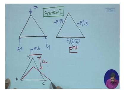
Now the external displacement go mostly to C dash. This is the displacement applied to joint B and this is D external.
