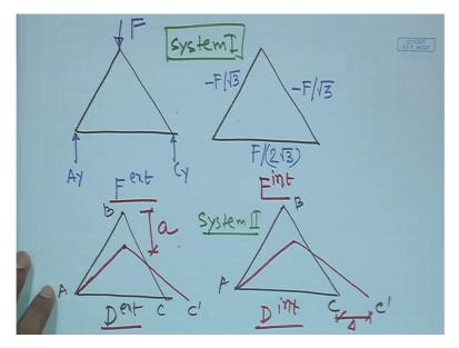
Now what principle of virtual work says? Principle of virtual work says that summation of F external into D external is equal to summation of F internal into D internal, okay.
