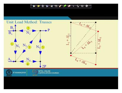
So DL1 is the change in length in member 1, DL2 is the change in length in member 2 and so on, okay. And just now we have seen the change in length can be obtained any jth member, the change in length can be obtained by this. Just now we have seen it, okay.
