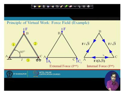
Now suppose this system we call system 1. The system 1 is essentially a force field which has the external force and the internal force, okay. Now these internal forces are due to this external forces, okay.
