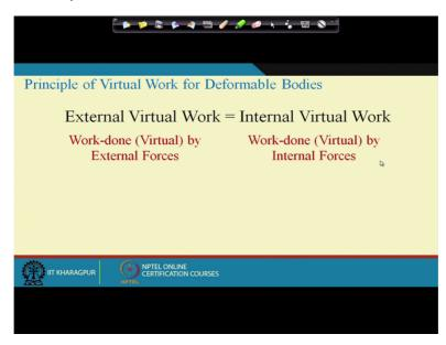
Then whenever we say the work done two important things are involved. One is the force and the displacement and then the associated force field is called as external force and suppose this is the associated displacement field which is D external and the force is F external. And similarly this is the internal force and this is the associated displacement.
