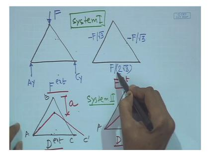
Now here it is given that there is no change in length in member AB and BC. Only change in length express in member AC. So this is F internal AB into D internal AB plus F internal BC into D internal BC plus F internal AC into D internal AC, right?
