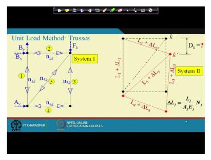
So system 1 is what? System 1 has a (ex) virtual force, external force and corresponding internal forces. So system 1 has the force field in this is virtual force field, okay. The external force is virtual and the corresponding internal forces we have that is due to the virtual external force. So this is system 1.
