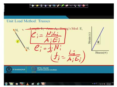
In a truss if the axial force is Ni and then Ai is called axial rigidity, okay. Because you see if Ai is more, then elongation is less and so if Ai is more means the member is axially rigid. So axial deformation in the member will be less. That is why Ai is called axial rigidity, okay.
