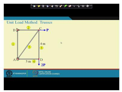
Now suppose this is the reactions and these are the external forces, okay. Now because of these forces suppose these members has internal forces like this, okay. Suppose these internal forces are denoted as Ni, okay.
