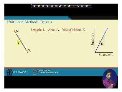
Now if the area of this member is a then what is the stress developed in this? Stress develop sigma is equal to Ni divided by Ai. That is the sigma, okay. Now then if sigma is this then what how this how this stress and strain are related? We know that epsilon is equal to sigma divided by E, right? So stress by Youngs modulus gives us strain.
