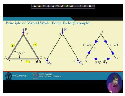
Now if you remember this is how we are showing the member force. This means that if it is shown in the member this means the member is in compression and if it is shown in member this means the member is in compression that is the sign convention we are following for member. Now so these are the forces in different members. Now this is the external force fluid and this is F external and this is F internal, okay.
