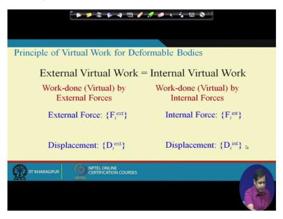
Now we have not made any statement whether the forces are real and displacements are virtual or the displacements are real or the forces are virtual. If you remember we said that we want to derive a general principle of virtual work and then see the principle of virtual displacement that we discussed in the last class. That is a special case of this general principle, okay. So in this case what is happening?
