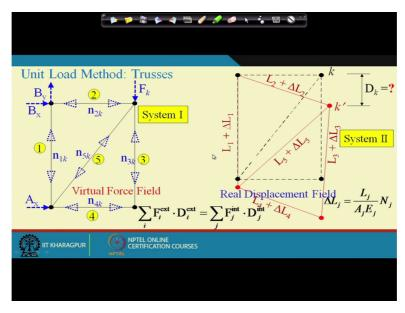
So external displacement will be this and internal displacement will be delta L1, delta L2 and so on. So (in) the external displacement is this and internal displacement will be delta Lj means it is the change in length in member J, okay.
