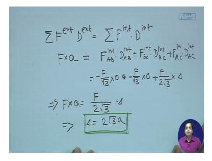
This now gives us a clue of developing a method. The method is now since any value of F this we can obtain the same delta. Give F is equal to 1, okay. So we apply F is equal to 1, get the F external D internal and then another system we have D external D internal which is conjugate to (ex) force field and then apply the principle of virtual work and get the corresponding displacement, okay.
