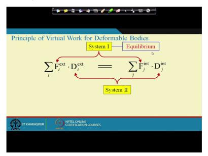
Now similarly what constitutes system 2? It is compatibility. Now if we give some displacement at any joint the member undergoes deformation and when the member undergoes deformation or the structure undergoes deformation all the members undergoes
