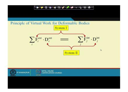
Now so what constitutes system 1? The equilibrium constitutes system 1. Because you see when we apply some external force in a structure some internal forces develop in different members and the summation of the internal forces should be equal to the summation of the external force, right? And that is equilibrium condition. So what constitutes system 1 is the equilibrium, right?
