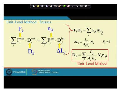
So we have just (demons) introduced unit load method. Probably when you demonstrate unit load method through some examples the concepts will be clear and that we will be doing in the next class. So next class what we will do we will determine the deflection of truss using unit load method, okay. (Refer Slide Time: 39:10)
