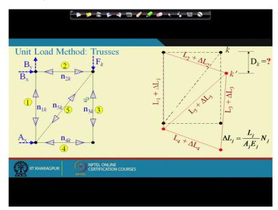
So n1K is the internal force in member 1 due to virtual load FK and similarly n2K is the internal force in member 2 due to virtual load FK and so on, okay. Now if we take this as system 1 and this as system 2, okay.
