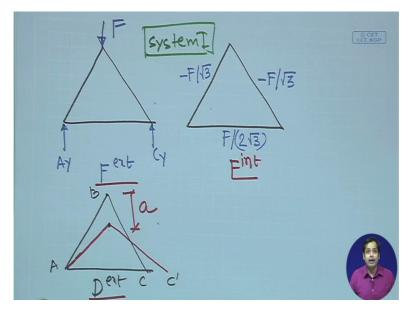
And then what is the corresponding internal? Internal will be, so this is A, B, C and this go to C dash and this distance is say delta, okay. And this is your (sys) D internal, okay.
