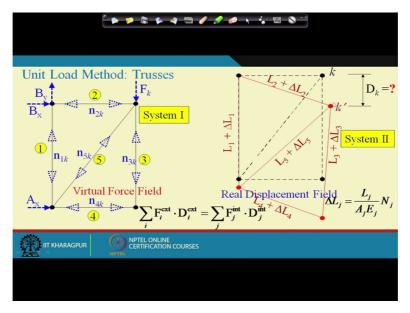
Now if we apply a displacement DK here then all the members will undergo deformation as delta L and the member 1 will undergo deformation delta L1, delta L2 for member 2 and so on if we apply a displacement delta K in member K in vertical direction, okay.
