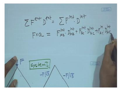
Now F internal is minus F by root 3 but this D internal is zero because there is no change in length AB, so this is zero plus this is again minus F by root 3 and this is zero because again there is no change in length in member BC. Then plus this is plus F by 2 root 3 into this distance is delta, okay.
