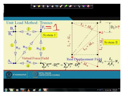
Therefore the force needs to be applied in vertical direction, okay. We apply a vertical force 1 unit load in the direction which we want to determine a displacement. Now this virtual load will generate some internal forces, okay. And then we also know the internal (for) elongation of this member by this.
