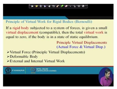
Now let us first understand what is virtual force and the associated virtual work, okay. Now suppose again consider the same object, then suppose for some load the object undergoes deformation like this and this deformation is the actual deformation.
