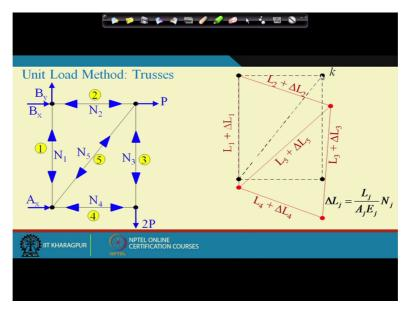
We have already seen method of joints and method of sections to find out internal forces in statically determinate trusses. Now what we want to do is we want to do the deflection. We want to find out the deflection of any particular joints or different joints and that we are trying to do through principle of virtual work. Suppose we want to find out what is the displacement of joint K. So this is DK. We want the displacement in vertical direction suppose, okay.
