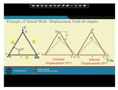
Now then this is called system 2. So system 1 is the force field and the system 2 is the displacement field. And we have two forces in system 1, external force and the internal force. And in system 2 we have two displacements, external and internal displacement, okay. And how the external forces and internal forces are related?
