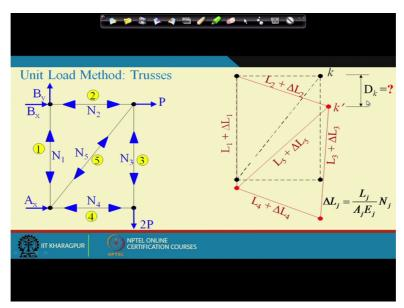
Now so our problem is finding DK. Now let us take the same truss and apply a virtual force at point K in the direction of DK, okay. Now because of this virtual force suppose these are the corresponding reactions.
