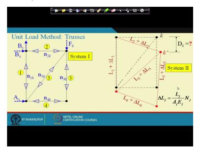
And the system 2 is the real (dis) displacement field, right? Now displacement field is real. So this is essentially principle of virtual forces where the force field is virtual and the displacement field is real, displacement field is real and the force field is virtual. Now if we apply the principle of virtual work considering these two systems and then what it says? This is virtual force field and this is real displacement field, okay.
