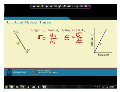
Then if the stress is this then what if the member is subjected to axial load Ni but this could be compression, this could be tension. Then what would be this strain epsilon i in this member. This strain epsilon i in this member will be, then if we substitute sigma here then what we have is Ni by Ai Ei. If the length of the member is Li then elongation in member Ei is equal to this strain multiplied by the length and this becomes Ni Li divided by Ai Ei. Ai Ni elongation is equal to this, okay.
