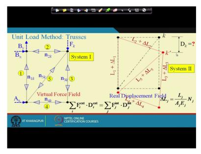
What we want to have to do is we have to apply a virtual force of 1 unit load in the direction. Suppose this is the displacement we want in vertical direction, right?
