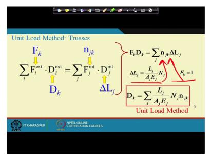
Why it is unit load method because the virtual force that are acting this is unit, okay. Now what unit load method says is? Unit load method says is just quickly let us see unit load method through, now suppose this is the structure and we have to find out what is the displacement in any particular direction.
