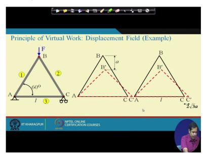
Now this is called external displacement because you are applying a displacement at joint B, okay, externally. And this is internal displacement. Internal displacement it means that this C-C dash this displacement this due to the change in length in member AC.
