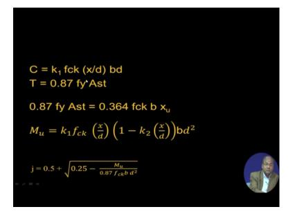
So coming to this on here this is a situation we are getting it here and as usual the C and T that one should be equal that C and T that will be equal so C and T we know and we know this one equivalent 0.87  $F_Y$  ast equal to 0.36 for f ck b  $x_u$  that parker one we can find out and then we can write down here  $M_u$  equal to  $K_1$  f-ck in x/d 1- $k_2$  x/d bd<sup>2</sup> I have taken all of them to the virtually who are your  $k_1$  fck x/d bd<sup>2</sup> that economy can take it here.
