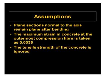
So let us click with the clicks are only and again we are having certain assumptions and those assumptions again you see that on the first assumption plane sections normal to the axis remain plane after bending the maximum strain in concrete at the outermost compression fiber is taken as 0.0035 so please note to this particular aspect that in working stress method we are totally silent only thing we have told that strain profile will be linear straight line that much only we have told.
