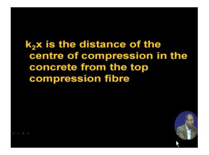
That is actually expert core portion ignored so only we are having compression concrete will take the compression and reason we take the tensile so  $k_2$  s is the distance of the center of compression in the concrete from the top compression fiber.
