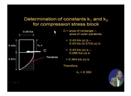
So we can find out that k1 and k2 this one area of rectangle that one- area of outer parabola so you can make this by culinary simple calculation then I can get it 0.364 f ck X into B so q1means 0.364.
