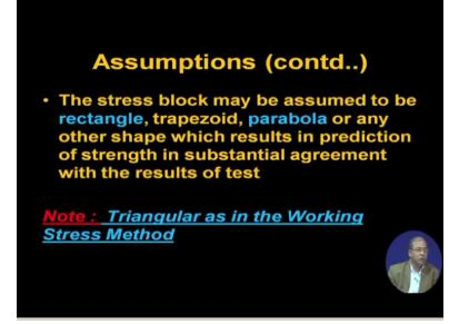
That to the stress block may be assumed to be rectangle trapezoid parabola or any other shape which results in prediction of strength please note the next one the substantial agreement with the results of tests so that means the code agrees that it will not exactly it will not match so that is why the code means you that a very wise lead it has told the substantial agreement so this why that is the one issue the understand that record on that at left on the substantial agreement.
