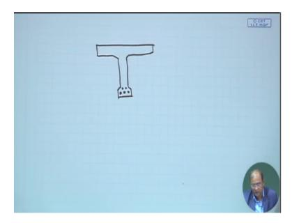
RCC t beam that one we let me tell this is the span dimension like this and we provide here that named reinforcement again longitudinal reinforcement whatever it is we provide there is your some main reinforcement, now let me show you one figure then it will be clear that how it comes. (Refer Slide Time: 13:10)
