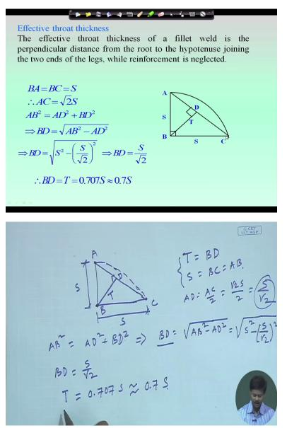
Now, (I will come to) now I will discuss about the effective throat thickness, as I told one is size of the weld. So if we see if we make a diagram that this is a size of the weld and (this the) this is root and from root to toe is a size of the weld and if size of the weld in different direction is same then we can write S or the minimum of that. Now extra deposits happens here, which is called enforcement and this extra deposit we provide to increase the efficiency of the joint.
