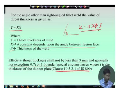
Now this is true for right angle triangle if it is right angle then fine we can find out this (()) (23:24) but what will happen about different angle means if it is joined like this, it is not right angle, right. So in this case what will happen, so that is defined in code that is in clause 10.5.3.1 of IS 800, it is told that the throat thickness will not be less than 3 mm and generally not exceeding 0.7t or 1t under special circumstances where t is the thickness of thinner plate?
