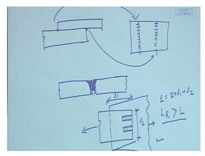
Let us come to here suppose 2 members are there and these are overlapped then when we are going to join this we need to join at the overlap portion and if we see in that plan we will see that these are say, these are welded. So this portion is this and this portion is this. So this type of welding is called fillet weld (())(8:10) means when 2 members are lapped together, 2 members are to be joint, in that case fillet member we can use and in case of fillet weld or I should say that
