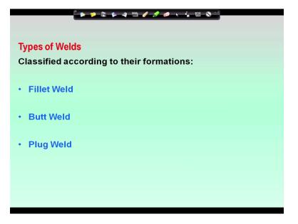
Now coming to type of weld, there are three types of weld we have, one is fillet weld. Fillet weld basically used when 2 members are lapped together.
