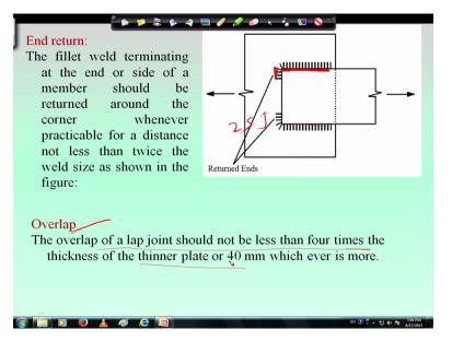
Let us come to that slide, this is called end return that means when the length of joint **is** is this then we have to provide a end return of this value and that is 2S. So this return, this is 2S, right. So if we provide here, the weld in this direction and this direction and if it is extended up to the corner then we have to extend up to 2S more, which is called end return and another thing we have to remember that is overlap.
