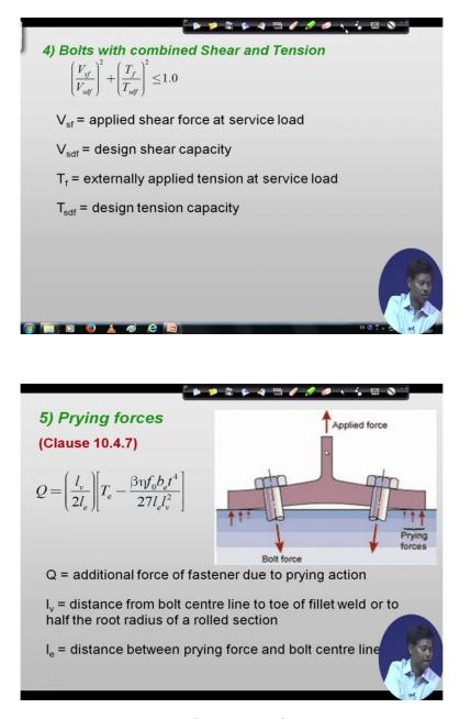
In clause 10.4.7 you will get the details of the prying force where it is mention that Q is equal to lv by 2le into Te minus beta into eta of be t to the power 4 by 27 le lv square, right. So this Q is the additional force (())(13:44) due to prying action and lv is the distance from bolt to center line to toe of fillet weld or to half the root radius of a rolled section that I will show in the figure.
