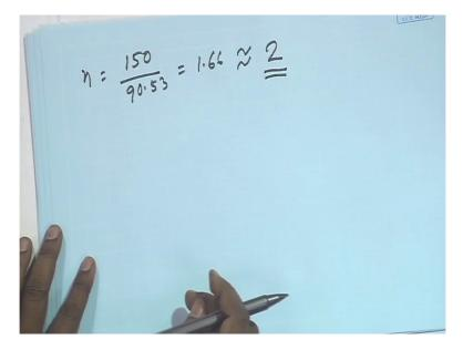
So number of bolt we can find out number of bolt will be 150 divided by 90.53 that means 1.66 that is 2, right. So 2 numbers of bolts require.
