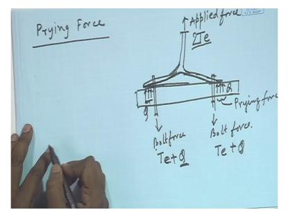
Now for high strength friction grip bolt, I will high strength friction grip bolt another force comes which is call prying force. This is very important prying force. Prying force is the additional force coming into picture in case of tension and if the deformation is allowed between two plates then prying force develops. Let me show through some figure, say one plate is like this which is attached with a say suppose I section, right.
