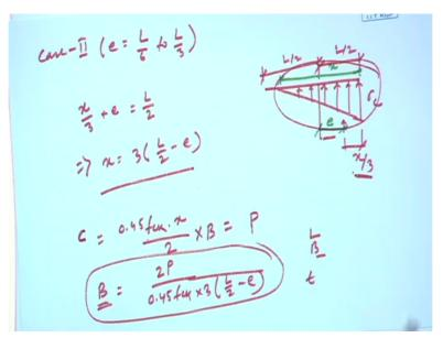
Now we will go to case 2, so case 2 is when e is equal to L by 6 to L by 3, okay. So in this case most part of the base plate is under compression with little or negligible tension on the remaining part. So if we see the diagram of the stress coming means pressure coming from the concrete pedestal to the base plate it looks like this this is sigma c and this is the neutral axis that means this is L by 2 and this is L by 2, right and this is x by 3, if this is x, this is x and this is e, okay.
