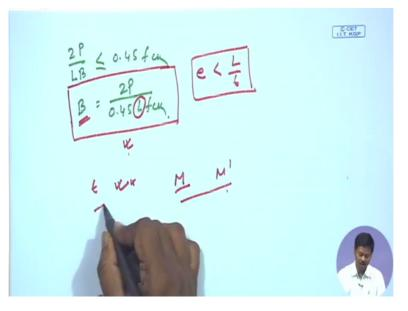
So the combined stress maximum combined stress is 2P by LB it should be less than or equal to 0.45 fck that means B should be equal to 2P by 0.45 L into fck, okay. So in case 1 when e is less than L by 6 what we can do we can find out the width or length of the base plate from this because we do not know what is the length and what will be the width so from the requirements from the dimension of the column we can approximately decide on the length
