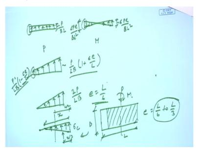
So different cases will occur here as we told that this is the uniform stress will come from the concrete block to the base plate of P by BL magnitude, right this will be P by BL magnitude. And another stress will be of this magnitude that is M by Z that is 6 Pe by BL square, right this value is 6 Pe by BL square and this value also same 6 Pe by BL square, right. So this is due to bending due to moment and this is due to axial load, right.
