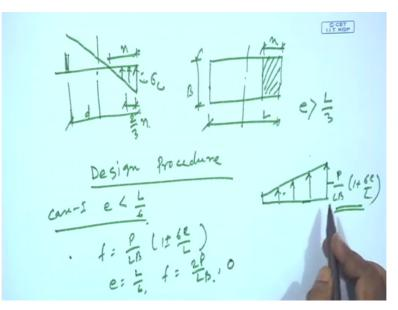
But if e is greater than L by 3 that means when the tension developed is substantial then the stress distribution will be like this so this is the neutral axis so this is this will be like this that means this will be sigma c and the neutral axis depth will be here n and at two third end the cg of this will be there, right and if bolt is provided here say in this position then we can
