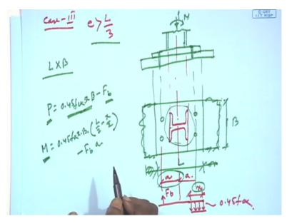
So next we will go to the third case, case 3 where e is greater than L by 3. So in third case if we see the diagram say this this is a column which is under axial compression and moment, okay. Now this is connected with base plate and then again with the concrete block, okay and this is connected with bolt anchor bolt here, right. So now if we see the plan this is the base plate length sorry width B and this is the sorry it will be from here so not this one, so this is
