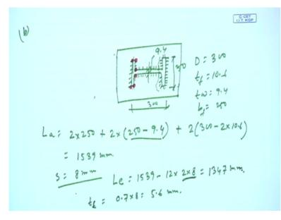
And for case b we have to design say for weld connection if we do as column end and base plate have not been machined for perfect bearing so the load from column will be transferred to the base plate through the weld connections. So if we see the weld connection so base plate is connected with the column so the weld connection throughout is periphery. Now I have to find out what is the total length available for welding and what is the required length to withstand that load, right.
