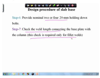
So after finding out the dimension of the base plate we will go to the step 6 where we will provide nominal two to four 20-mm holding down bolts just to hold the the column in proper position on the base plate, right this is true of axial axial compression load however for moment we have to design that. If moment is there then we need to design that how many bolts are required that will come later.
