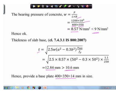
Then the bearing pressure of concrete we can find out that is w is equal to P by LB, so P is 1200 kilonewton and length is 400, width is 350 so the bearing pressure of concrete we can find out 8.57 which is less than 9 9 is the bearing strength of the concrete that is 0.45 fck. And then we can find out t that is thickness and that will be is coming 12.84 which is greater than the tf thickness of flange as 10.6, so we can provide a base plate of 400 by 350 by 14 mm size, okay.
