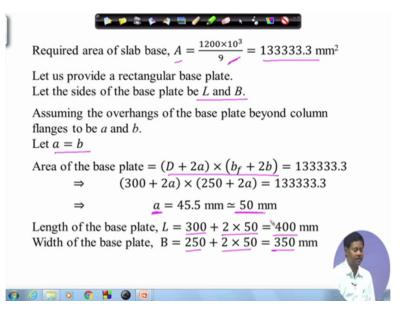
After that we will find out the area of the slab base that is A is equal to P by 0.45 fck, so the required area of slab base can be found and if we provide a rectangular base then say side of the base be L and B and if we assume the overhang of the base plate beyond the column equal that means a and b are equal then the area of the base plate we can make equal with this to find out the overhang position of a.
