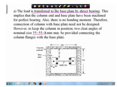
So once we find out the size of base plate now we will connect the base plate with the column. So there are two cases one will be load when it is transferred to the base plate by direct bearing so in this case as there is no moment so we can provide a nominal number of bolts and a nominal size of the cleat angle, so here we are providing nominal size of the cleat angle as 55 by 55 by 8 and two numbers of bolt of 20 mm diameter, right.
