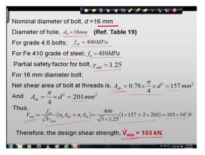
So if we see now that nominal diameter of bolt was given as 16 mm, so hole diameter will be d0 will be 16 plus 2, because as per table 19 the clearance of the bolt for 16 mm diameter will be 2 mm. So the whole diameter will become 18 mm and for 4.6 grade bolt we know fub the ultimate stress of bolt will be 400MPa and for Fe 410 grade of steel fu we know fu is the ultimate tensile strength of the plate that is 410MPa and partial safety factor from table 5 we can find out as gamma mb as 1.25.
