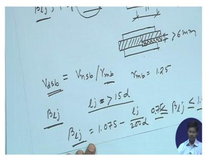
Now let us come to the reduction factor how do we calculate beta lj this is reduction factor due to long joint. So long joint means what long joint means if this length of joint become more than 15 times of nominal diameter of the bolt if this length of joint become more than 15 times of nominal diameter of the bolt then we can calculate beta lj as this 1.075 minus lj by 200d.
