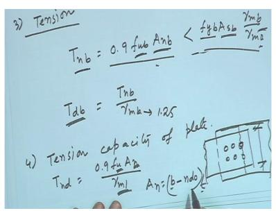
Next will come bolt in tension, so for tension we can calculate the nominal capacity of bolt in tension as Tnb is equal to 0.9 fub into Anb and it has to be less than fyb Asb into gamma mb by gamma m0, right. So Tnb we can calculate from this formula also we will calculate this and we have to check that Tnb is becoming less than this otherwise you will calculate this value.
