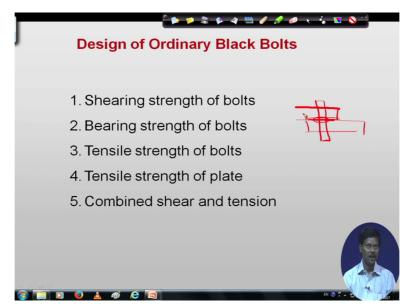
Now for designing of ordinary black bolt we will see that what are the failure criteria and from that failure criteria (what are the shearings) what are the strength like it may fail due to shear. We know the black bolt when we are going to design suppose the plates are here and another plates are connected here and we are designing a bolt then there is a chance of failure in this shear plane.
