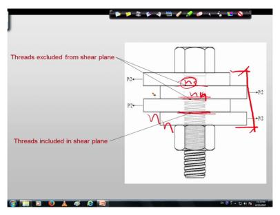
That means if we go next page you will see here the entire if we see that entire bolt grip is this much sorry this is the entire bolt grip. Now say for example in this case the thread included in shear plane is this one this shear plane is included by that threads. Now the threads excluded in shear plane is this one or this one. So this is nn and nb, so nn and nb we can define as nn as number of shear planes without thread intercepting the plate.
