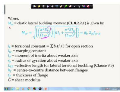
So our next step is to find out the value of Mcr, which is given through this expression Mcr. This is available in the code in clause 8.2.2.1 the details are given, so from that the value of Mcr can be found. Now where here the different parameters are defined like It the torsional
