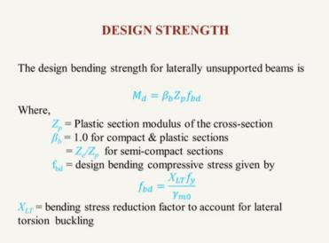
So if we see the design bending strength, which we can write as Md is equal to beta b Zp into.
