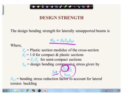
So the things whatever we have discussed, I am just quickly going through this power point that is first we can find out design strength. So the design strength for lateral torsional buckling has been calculated as per the codal permission and I am very quickly going through this formula, which I have written in hand. So you can see that first we have to find out, the design bending strength for laterally unsupported beam from this formula that is Md is equal to beta b Zp Fbd.
