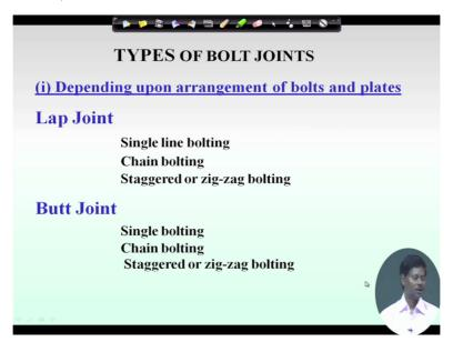
Now coming to depending upon arrangement of bolts we can see that we have two type of joint we can make one is lap joint another is butt joint. So in case of lap joint we have we have seen earlier also we can make a single bolting, chain bolting and staggered bolting. And in case of butt joint similarly we can have single bolting, chain bolting and staggered bolting. So coming to the different bolting pattern first let us come to the chain bolting.
