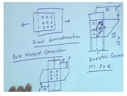
Say for example direct shear connection, in case of direct shear connection we can see that if two plates are overlapped together then this type of connection is called direct shear connection. So when such type of condition will come we will design the bolt accordingly due to shear it may fail so we can find out the strength of the joint.
