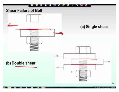
Say first let us come to a failure which is called shear failure, so this is a shear failure for different case with single shear and double shear. Now if you see for single shear that means only one shear plane is there between two plates only one shear plane is there, that is why it is called single shear failure so how the failure may occur that due to shear of the bolt at this point it may fail.
