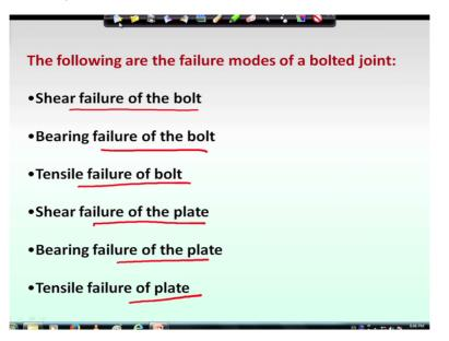
Now we will discuss about the different type of failures because when we are going to design a bolt, when we are going to find out the strength of a bolt, or strength of the connection as a hole we have to find out what are the type of failure may occur and to arrange those failures what are the mathematical equations are developed and how we will calculate the strength.
