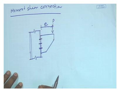
Then moment shear connection, in case of moment shear connection that is suppose say column may be I section and we have a bracket and this is connected in this way. So it is connected in this phase, right so bolting will be in this way. So in this case moment and shear will be developed this is e, this is P, so moment and shear will be developed so this is called moment shear connection.
