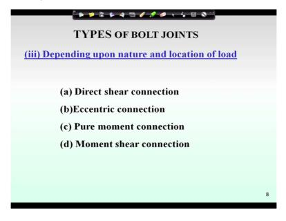
Now depending upon nature and location of load we also can find out different type of connections like direct shear connection, eccentric connection, pure moment connection and moment shear connection, so four type of shear connection we can see depending upon the nature and location of load. Let us see how it looks.
