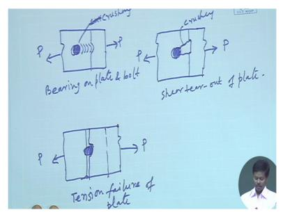
Now we will see bearing on plate and bolt, bearing failure how it happens. So if we see the two plates if it is connected and this is a bolt then due to bearing on plate it may fail that means it may fail like this is crushing. So this is one type of failure which is called bearing on plate bearing failure, plate and bolt.
