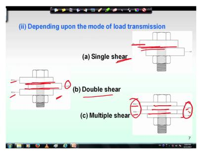
So the single shear when it comes here we see when the two plates are joint together this is one plate, another plate and it is joint through bolt then only one shear plane is there that is why this is called single shear and in this case if we see that one shear plane is here where it may fail another shear plane is here where it may fail, therefore this is called double shear.
