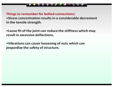
Now we have to remember certain things for a efficient connection using bolt that is one is the stress concentration results in a considerable decrement in the tensile strength so we have to try to avoid the stress concentration. Then loose fit of the joint can reduce the stiffness which may result in excessive deflections. So that has to be taken care that means we have to tighten the bolts properly so that the loose fit does not occur and joint does not get reduced instantly.
