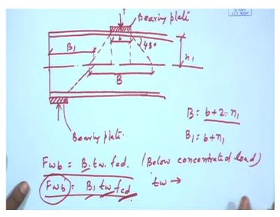
Now web buckling strength will we will like to calculate. So for calculation of web buckling strength we need to find out how the baring plate is going to be provided to minimize the web buckling means to reduce the web buckling, say for example, if a member is subjected to concentrated load at certain point, say concentrated load p is there and this is called bearing plate bearing plate.
