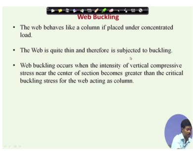
So as the web behaves like a column, therefore the web strength we have to calculate the strength means the, but it will compressive strength we have the center of the web we have to calculate and then we have to check whether it is safe or not.
