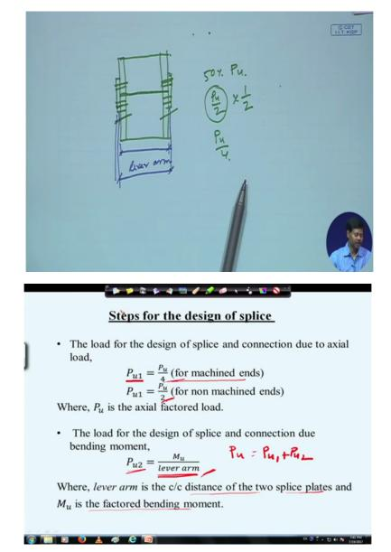
So this is what we have to remember, now how to find out the process. So here we will see the load for design of splice and connection due to axial load we can consider as Pu1 as Pu by 4 for machine end. Why Pu by 4 let us see if we see here design, if columns are spliced at a certain points then we know this has two plate right in two sides, so these are to be connected by the bolts or welds due to certain load.
