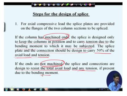
Now let us see what are the steps we need to follow so that we can design the splice properly. So if we see the steps the steps are made based on the column positions and in the means considering the column positions we have made the steps in the following order. Say first so for axial compressive loads the plates are provided on the flange, flange is of the two columns sections to be spliced.
