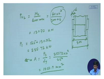
Load on splice due to moment which is we can say as Pu2 that will be Mu by lever arm. So we have to find out lever arm right so Mu is given which is 40 into 10 to power 3 Mu was given 40 kilo Newton metre, so 40 kilo Newton into 10 to the 3 to make it kilo Newton millimetre by lever arm, lever means 300 is the depth of the I section + 6 mm is the plate thickness. If we assume plate thickness, splice plate thickness as 6 then we can consider 6.
