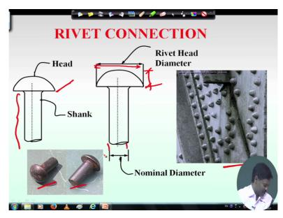
Now coming to Rivet Connections we know rivets are inserted in the plates to join together different plates and by adding heat we can insert the rivet like this so this rivets can be inserted a typical rivet joint is showing here where different members are connected to plate by riveting and in the parts of rivet which is there is head, this is this part is called head and this part is called shank.
