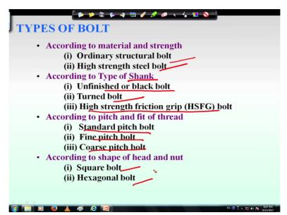
Now coming to types of bolt, what are the types of bolt, we can classify the bolts in different way, one is according to the material and strength according to material and strength we can classify this as ordinary structural bolt and high strength steel bolt, this two type we can make.
