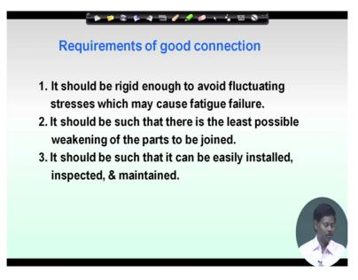
Now let us come to the requirement of good connection, what is good connection basically good connection mean it should be such that it can easily be installed, inspected and maintained that is one thing, then it should be such that there is the least possible weakening of the parts to be joined and it should be rigid enough to avoid fluctuating stresses which may cause fatigue failure. So this thing has to be kept in mind.
