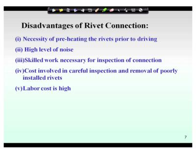
But it has lot of disadvantages also, what are the lot of disadvantages let us see, one is the necessity of pre-heating the rivets prior to driving is required so that is very important, then another thing is that high level of noise is created. So at the site where construction is going on, high level of noise can be created. So generally we nowadays we try to avoid this noise.
