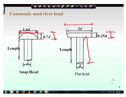
Now commonly used rivets are like snap head snap head where the head dimensions are fixed head dimension means in terms of diameter of the shank if diameter of shank is d then we can consider that that the diameter of rivet head is 1.6d and the height of the rivet head is 0.7d, so with different height and diameter different type of heads are snap means rivet heads are available and its name are different, I have just given here two type of rivets one is snap head, another is flat head.
