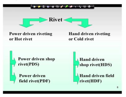
Now coming to different type of rivets we can see that one is power driven rivet another is hand driven rivet, there are two types of rivets. Power driven rivet is called hot rivet and hand driven rivet is called cold rivet, again in power driven rivet we have two types one is called power driven shop rivet, another is called power driven field rivet. And similarly for hand driven rivets hand driven shop rivet and hand driven field rivets are available.
