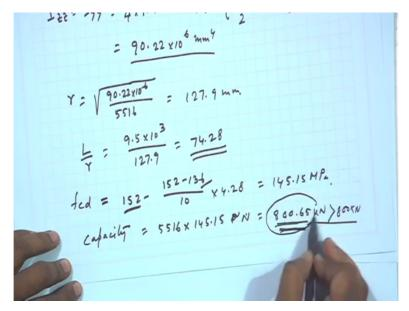
Now from table 9c I can find out the actual fcd earlier we got the required fcd now from the actual dimension actual spacing of the members we can find out the design compressive stress fcd as 152 minus 152 minus 136 this can be found from table 9c corresponding to L by r as 70 it is 152 and as 80 it is 136, so if we interpolate we can find out the fcd value as 145.15 MPa.
