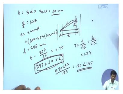
Now I have to find out the length of the lacing flat. So to find out length of lacing flat and the depth width of the lacing flat we have to use certain connection, so that can be found that whether we are going to use the weld connections or bolt connections. So there are two option in this case let us assume 20 mm diameter grade of 20 mm diameter of bolt of 4.6 grade we are using.
