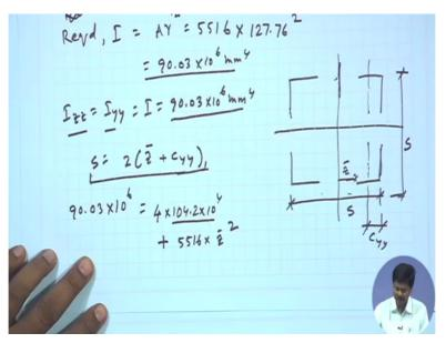
So if required r is this then we can say that required moment of inertia required moment of inertia I is equal to Ar square, now A is fixed, A already we have fixed as 5516 because the section size is fixed only the spacing between size is not fixed so into 127.76 square, okay. So 90.03 into 10 to the power 6 millimetre to the power 4 so this is the required moment of inertia about (I-I or z-z) y-y and z-z.
