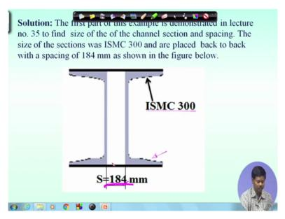
So same example has been considered here and in lecture 35 we have seen that how to calculate the spacing between two members and how to decide the section size that has been
