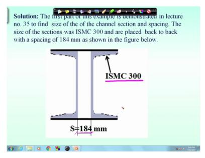
So if we recall the design example provided in lecture 35 we can see that we obtained ISMC 300 channel section and having a spacing between these two as 184 and channels were placed back to back. So this is what already we have calculated. Now we will calculate the forces coming on lacing and the dimensions of lacing.
