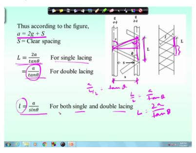
Next is so a will become basically S plus 2g, where S is the clear distance and g is the gauge distance. Now we have to find out the length length of length between two lacing, so which is called spacing clear spacing sorry spacing between two lacing, right. So how do we find out the length length means this one, so we know this value a, a means the distance between bolts so if we know a then we can find out the value of this, right.
