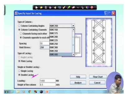
Here channel opposite to each other has been consider, here another option has been consider that is if we consider double lacing system then how the orientation will be done that has been shown here. So the program can take care the design of double lacing system as well, right.
