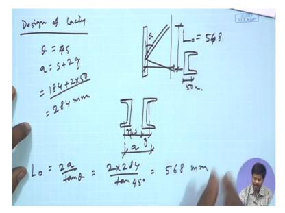
Now we will come to the design of lacing system, so coming to design of lacing first we will find out the angle of lacing. So what should be the angle of lacing, so that has to be decided, right. So so in first step we have seen that we have to assume the angle of lacing, so here we can assume say angle of lacing theta as 45 degree, right and for this channel section the gauge distance was given in SP: 6 it is 50 mm, right.
