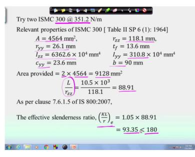
So next higher section is ISMC 300, so if we choose ISMC 300 then we can see the relevant properties of the section as the cross-sectional area of individual section is this, ryy is this, rzz is this, remember that rzz is increasing from the earlier one also A is increasing, so load carrying capacity will definitely increase. Then Izz is this, Iyy is this and Cyy, b from table 2 of SP: 6 we can found as this.
