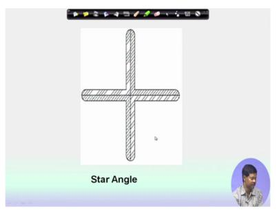
This is an another type of built-up member which is consisting of 4 angles which is called star angle.
