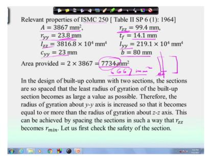
So if we provide 2 ISMC 250, let us see what will be the combined area and its properties. So if we see that relevant properties are given here that one is the for ISMC 250 area is 3867 millimetre square, ry is 23.8 and rz is 99, so here you see rz is much greater than ry. So if we use a single section single section then it will buckle about weaker axis that is y-y axis. So to resist that we use 2 section, right.
