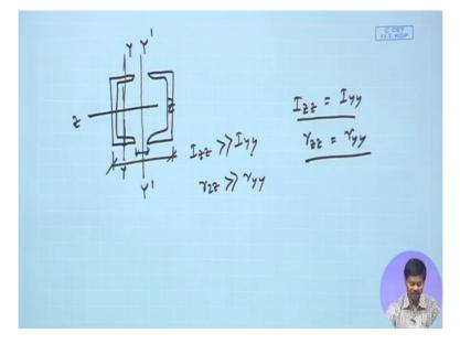
Say for example if we consider a channel section as a compression member, then we know if this is z-z and if this is y-y axis if we consider, then Izz is much higher than Iyy, right or rzz is much higher than ryy much higher than ryy. Therefore the chances of buckling about y-y axis will be much earlier than about z-z axis. So if we provide built up member then what we can do we can increase the radius of gyration by by providing another member and with a certain spacing.
