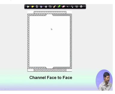
Next is channel section when facing face to face this way also we can provide a built-up member.
