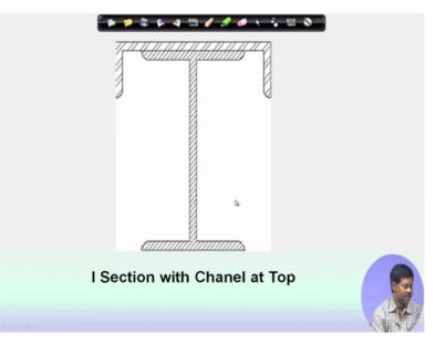
Then I section with channel section at the top as per the requirement, sometimes we see the requirement and according to that requirement we may have to provide that I section with a channel section at the top.
