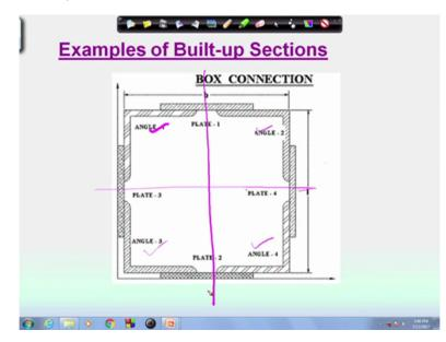
Now now examples of built-up member if we see, here we can see that we can use 4 angle section 4 angle section and to make a box type of cross section by the use of certain tie plate which is called generally lacing or battening that I will come later. So this is one example where we can use built up section to increase the Ixx and Iyy of the section.
