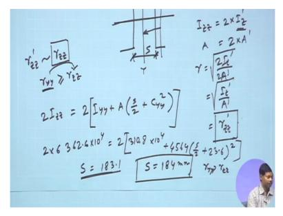
So from this I can find out value of S as 183.1 that means if I put S the spacing between two section as 183.1 then equal strength can be achieved. So we can provide say S is equal to little higher say 184 that means ryy be little higher than rz, right. So the spacing between these two members should become 184.
