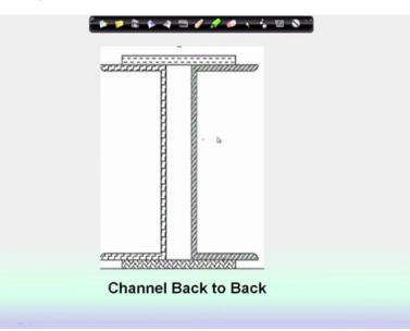
Another different type of built-up members are used another example is that when two channel sections are placed back to back, then also the built-up members means are connected with the lacing or battening member, so this is one example. (Refer Slide Time: 5:19)
