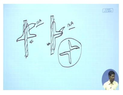
So angle sections may be provided like this, say suppose two angle sections I want to provide. Now that may be possible if I use two angle section on the opposite side of gusset plate, this is one way we can make, this is gusset plate, right otherwise we can arrange the angle sections as like this also that means in same side of the gusset plate this will be. So this
