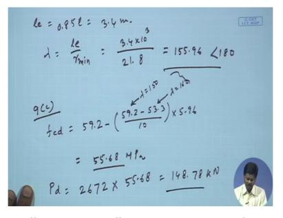
Now let us come to effective length so effective length will be same for this case also le will be 0.85l, so 3.4 meter and lambda I can find out slenderness ratio as le by r, r means r minimum, so this will become 3.4 into 10 cube to make it millimetre by r minimum is 21.8, so this is becoming 155.96 newton per millimetre square which is less than 180, right. So this is okay, from slenderness ratio point of view it is okay.
