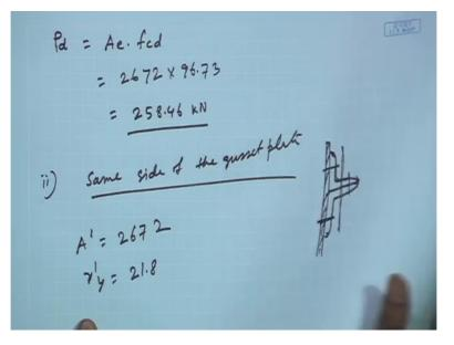
Now the strength design strength of the member now I can find out that will be Ae into fcd, so if I put those value of Ae and into fcd, Ae is 2672 which is the area of two angle section into 96.73 is the fcd value. So this will become 258.46 kilonewton, right. So design strength of the member can be found as 258.46 kilonewton.
