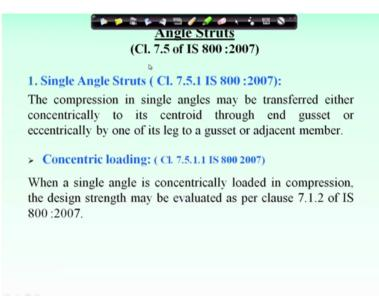
Now this compressive load may act concentrically on the angle section or may act through its one leg which will be eccentric and this angle section calculation means the strength calculation of such type of angle sections are given in code in clause 7.5 of IS 800:2007. Now in clause 7.5.1 of IS 2007 it is told that the compression in single angles may be transferred either concentrically to its centroid through end gusset or eccentrically by one of its leg to a gusset or adjacent member.
