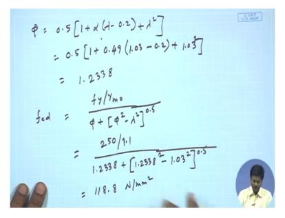
So as lambda e value has been changed the phi value will be changed because phi value depends on the lambda e, so phi value I can find out that is we know 0.5 1 plus alpha into lambda minus 0.2 plus lambda square. So putting the value of alpha and lambda in this equation, alpha is 0.49 and lambda is 1.03 if I put this value then the value of phi I can found I can find as 1.2338.
