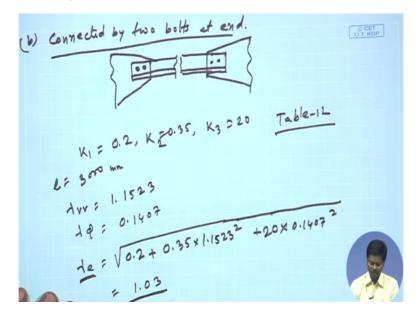
Now the same calculations will be done when the two sides are calculated by two bolt for the same case and let us see how the strength is going to vary from earlier case. So two bolts means if I see this member if two members are connected if these members are connected
