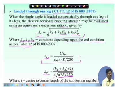
However if this is not concentric then we have to go for another clause which is given as a clause 7.5.1.2 when loaded through one leg, if the angle section is loaded by the axial
