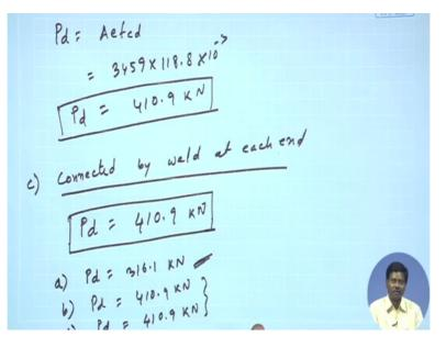
So the Pd value I can find as Pd is equal to Aefcd that will be 3459 into 118.8 into 10 to the power minus 3 to make it kilonewton. So this will become 410.9 kilonewton. So for second case the design strength of the compressive member will become 410.9 kilonewton.
