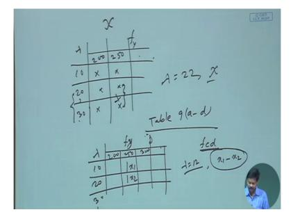
So in table 9 (a to d) we can see that for different value of lambda and for different value of fy yield stress, we can find out the value of fcd. Say for example say 10, 20, 30 like these lambdas are varying and fy is say 200, 250, 300 like this it is varying. So for a particular value of lambda we can find out the value of fy and then from the table 9 a, b, c or d according to the buckling class we can find out the value of fcd fcd value, say for example this is x1, this is x2 for 10 and 20.
