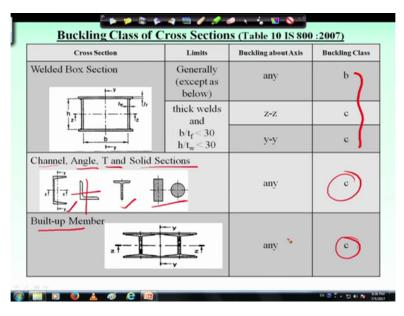
Now coming to weld box section, here also buckling class has been defined. Similarly I am not going into details we can means we can find out in the code, in table 10 only thing I want to mention that when we are using channel section, angle section, T section or some solid section, solid section means rectangular section or circular section then the buckling class will be c about any direction about any direction, say for angle about y-y axis, about z-z axis it will be c for both the direction.
