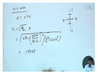
Similarly I have to find out the design compressive stress about y-y axis about y-y axis because the member may fail if this this is the I section it may fail about z-z axis, it may fail about y-y axis. So the about weaker section it will fail so we have to find out which one is the weaker one.
