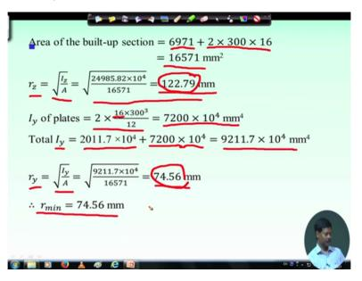
Similarly we can find out Iyy also, now the area of the built-up section also we can find out, area of the section was 6971 that is rolled section area ISHB 250 and area of the plate is 300 into 16 into 210. So total area of the built-up section will be 16571 millimetre square. So we can find out, the radius of gyration about z-z axis that is Iz by A square root of that, so after calculation we can find out rz as 122.79 millimetre.
