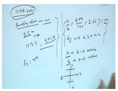
So now from this cross sectional properties we can find out h by b, here h by b is 400 by 140 which is becoming 2.86 and it is more than 1.2 and thickness of flange tf is 16 mm which is (more) less than 40 mm. Therefore from these two we can find out the buckling class as per
