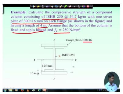
Another example we will go through quickly similar example but this is a built-up section, this example we will go through. Here we need to calculate the compressive strength of a compound column consisting of ISHB 250 with one cover plate on each flame of 300 by 16 as shown in the figure and having a length of 4 meter, assume that the bottom of the column is fixed and top is hinged, so boundary conditions are given and fy is 250.
