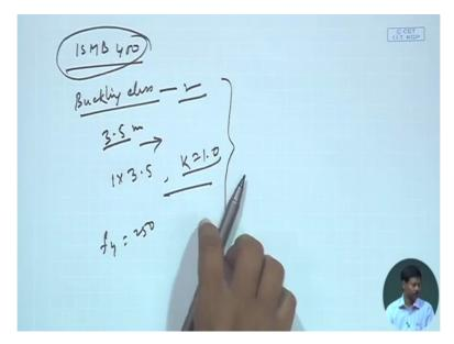
That means from this what we could see that ISMB 400 members are used. So from this we can find out what is the buckling class where ISMB 400 we know the thickness of the member that means thickness of the flange, width of the flange and the depth of the cross section those things we know, so from this we can find out the buckling class then another thing we can find out that is the slenderness ratio, slenderness ratio here the length is given 3.5 meter.
