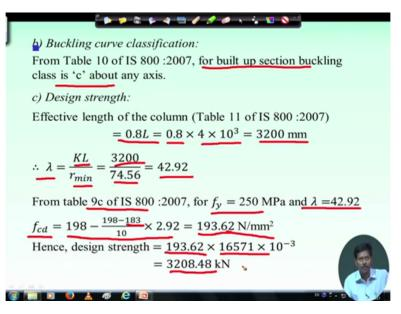
So now we will consider r minimum and we will find out the radius of gyration, ok. Now radius of gyration we can find out lambda as KL by r minimum and here KL we have to find out, now KL is as per the distant condition it will be 0.8L, so 0.8 into 4 into 4000 so 3200 millimetre will be the effective length of the column. So effective length of the column is 3200 and r minimum is this, so lambda will be 42.92, right.
