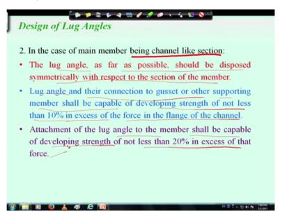
Then in case of main member being channel section, so earlier we have consider angle section main member, here we are considering main member as channel section if it is then we should remember that the lug angle, as far as possible should be disposed symmetrically with respect to the section of the member because in channel section channel section it shall be the symmetric. So lug angle should be provided at the top and bottom in a symmetric way.
