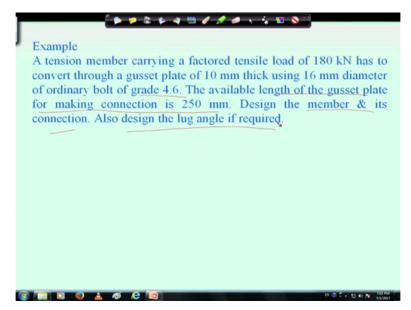
So here you see this is given that a tension member carrying a factor tensile load of 180 kilonewton has to convert through a gusset plate of 10 mm thick using 16 mm diameter of ordinary bolt of grade 4.6. The available length of the gusset plate for making connection is 250 millimetre. Design the member and its connection. Also design the lug angle if required. So here what we see the connection length is limited, so here connection length is limited to 250 mm available length is 250 mm.
