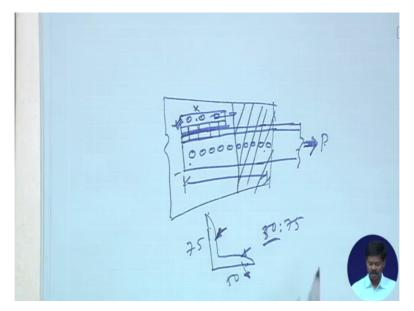
That means if an unequal sections are used say suppose this is 75 and this is 50, then load to this leg and load to this leg will be with the ratio of 50 is to 75. So less load will be shear by this angle and more load will be shear by this angle. So with this ratio it will be shear, this is what codal provisions says.
