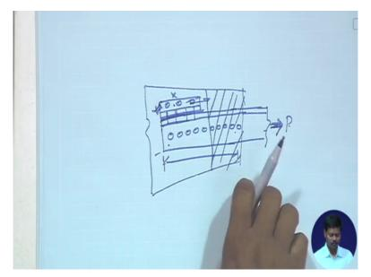
I can show a diagram say suppose a angle sections are connected with a gusset plate, right suppose this is an angle section. Now if this angle section carries a huge load huge load if it carries then I need lot of number of bolts and this is how it increases the length of the gusset plate say suppose this is the length of gusset. Now to save the material sometimes we may be able to reduce this length by putting an additional angle with the with connected with the main angle in this directions.
