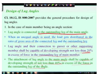
So before going to design I am going to provide the codal provisions once again I like to discuss the details about the lug angles like ok. In clause 10.12, in IS 800:2007 here it provides the general procedure for design of lug angle. So when we will be going for designing we have to keep in mind these codal provisions. It is two type one we can provide angle section, another is we can provide channel section. The main member may be angle or main member may be channel sections.
