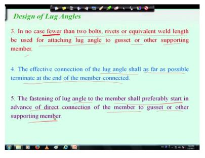
And then other few criterias we have to remember that is in no case fewer than two bolts, rivets or equivalent weld length be used for attaching lug angles to gusset plates or other supporting member. That means when we are attaching the member with the lug angle and lug angle with the gusset plate atleast two number of bolt or rivet has to be provided, right.
