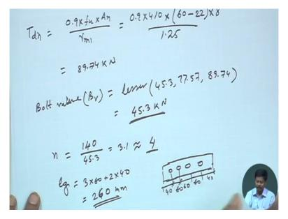
Now strength of angle for pitch we have to also find out that is Tdn that is we know 0.9 into fu into An by gamma m1. So if I put the value it will be 0.9 into fu is 410, now now An An will be per pitch if we consider so 60 is the pitch and diameter is diameter hole of hole diameter of the bolt is 22 into thickness is 8, right by 1.25. So strength of angle per pitch length we can find out this will become 89.74 kilonewton, right.
