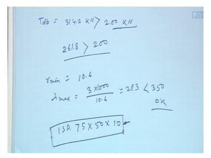
That means the Tdb value is will become 314.2 kilonewton and that is greater than 200 kilonewton, ok. So here the design tensile strength of angle we are getting lesser of these three Tdg, Tdb and Tdn that is 261.8 kilonewton and the external load is coming 200 kilonewton, so this is absolutely ok so we can go ahead with this section. Now I have to go for slenderness ratio check.
