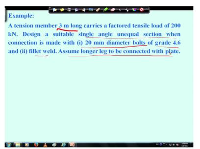
So problem is like this a tension member 3 meter long carries a factor load of 200 kilonewton 200 kilonewton load is the Tu value, 3 meter long effective length is 3 meter and design a suitable single angle unequal section, so it has been told you have to use single angle not double angle and unequal section, right when connection is made with 20 mm diameter bolt of grade 4.6 and fillet weld. Assume longer leg to be connected with plate, right.
