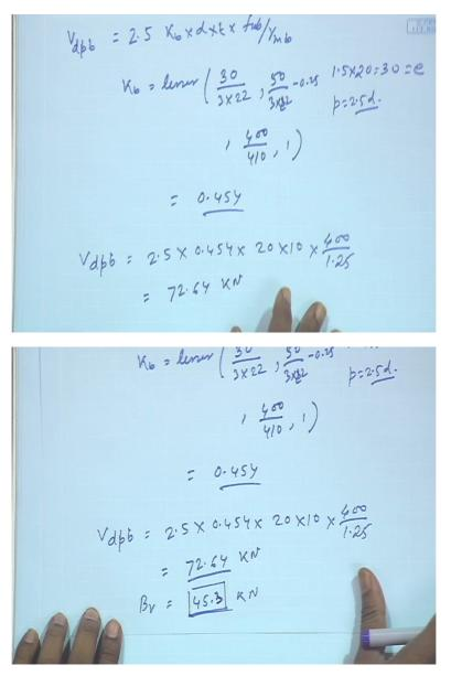
Again bearing strength of bolt Vdpb if I say it will be 2.5 Kb into d into t into fub by gamma mb, right. Now we have to find out the Kb value Kb will be we know lesser of e by 3d0, e we can consider 1.5 into d so 30 so e by 3d0, d0 is 22 and P by P I can consider this is e, P we can consider 2.5d that means 2.5 into 20, right so it will be 50, so 50 by 3 into (32) 22 minus 0.25, like this then (fu by) fub by fu then 1, so lesser of this is coming as 0.454, right.
