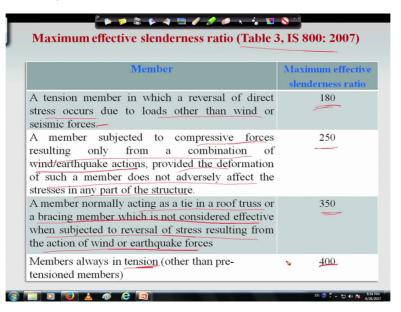
So the slenderness value slenderness ratio value are given in table 3 of IS: 800-2007, if we see that we will see that when the tension member has reversal of direct stress due to loads other than wind and seismic it is 180 180, right.
