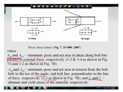
Now while calculating block shear failure we have to know the Avg and Avn value how to calculate this is given in the code in figure 7 it is mentioned that this will be the minimum gross and net area in shear along bolt line parallel to the external force, that means 1-2 and 3-4 in plate and 1-2 in angle.
