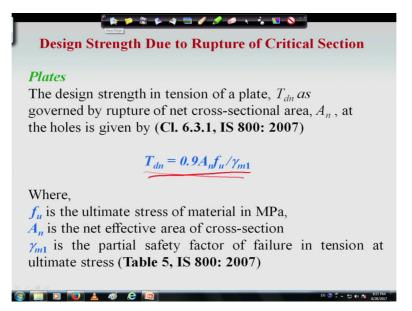
Then design strength due to rapture of critical section if we see we can find out that Tdn is equal to 0.9Anfu by gamma m1, where fu is the ultimate stress of material and An is the net effective area of the cross section and gamma m1 is a partial safety factor. So for plate simply we can find out Tdn as 0.9Anfu by gamma m1.
