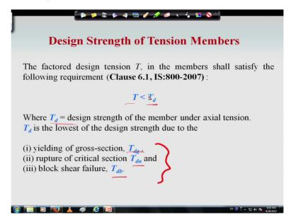
So if I see quickly the design strength calculation for tension member we have to see that these three criteria we have to calculate one is yielding of gross section, then rapture of critical section and block shear failure and the least of these three will be the design strength of member and which should be means the factor design tension should be less than that design strength.
