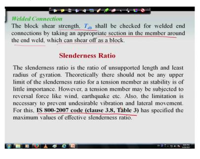
In case of weld connection the codal provisions says that the block shear strength Tdb shall be checked for welded end connections by taking an appropriate section in the member around the end weld, which can shear off as a block so that we have to take care. And in case of slenderness ratio the maximum (())(33:27) slenderness ratio are given in table 3 of IS: 800-2007 and in clause 3.8 it is mentioned.
