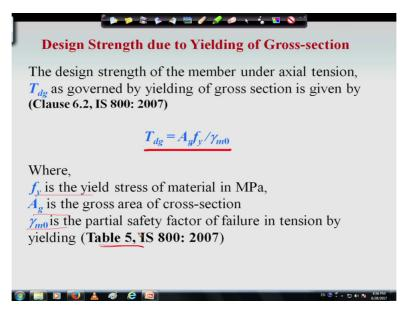
So to find out this we have to calculate the design strength due to yielding of gross section, that we can calculate this is the Tdg is equal to Agfy by gamma m0. Now Ag is the gross area of the section and fy is the yield stress of material and gamma m0 is the partial safety factor
