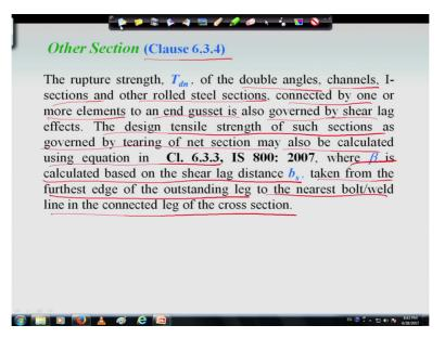
For other section other sections we can see here which is given here that is written in clause 6.3.4 which I have represented here that is the rapture strength Tdn of the double angle because earlier we have calculated for single angle, for double angle channels I-sections and other rolled steel sections connected by one or more elements to analysis end gusset is also governed by shear lag effect.
