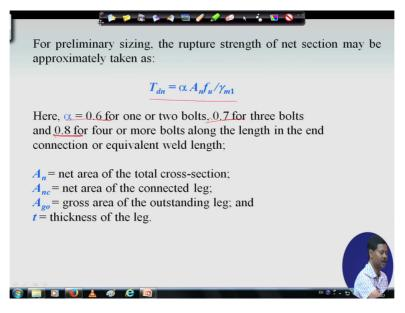
And for preliminary sizing we can find out the rapture strength approximately as this Tdn is equal to alpha into Anfu by gamma m1 and this alpha value has been given in the code as 0.6 for one or two bolts, 0.7 for three bolts and 0.8 for four or more bolts along the length in the end connection, so this is how we can approximately find the Tdn value.
