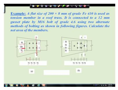
Now another problem we will go through that is a comparison between chain bolting and zigzag bolting, this is the problem. Say a flat size of 200 by 8 mm of grade Fe 410 is used as tension member in a roof truss. It is connected to a 12 mm gusset plate by M16 bolt that means 16 mm diameter bolt of grade 4.6 using two alternate methods of bolting as shown in the following figure. Calculate the net area of the member.
