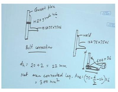
So to start with we can see that first case we can consider that a gusset plate is connected with an angle section of ISA 75 by 75 by 6 with a bolt, right. So this member size is (7) ISA 75 by 75 by 6 and this this is gusset plate and this bolt is M20 grade of bolt with 4.6 grade, so this is one case.
