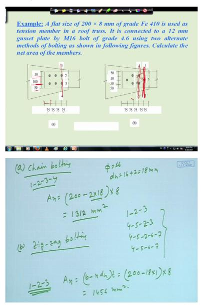
So for chain bolting we can find out the net area along line 1-2-3-4 that will be simply An is equal to 200 minus 2 into 18. Here nominal diameter of the bolt is 16 so bolt hole will become dh will become 16 plus 2 that is 18 mm, right. So the along this line 1-2-3-4 two bolts are there therefore the reduction will be 200 minus 2 into bolt hole bolt diameter into the thickness thickness was given as 8 mm. So after calculating we can find out this is 1312 millimeter square.
