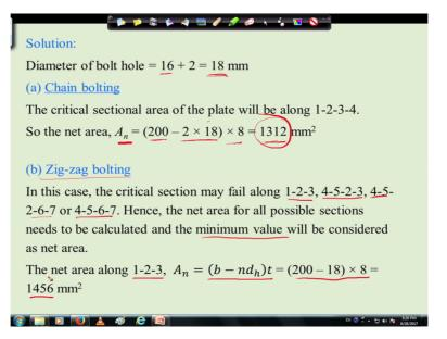
So if we go the solution we will see for chain bolting the net area will be 200 with minus the hole area into thickness so 1312, right.
