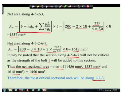
Similarly if I go next 4-5-2-3 we can find out the net area that will be b minus ndh plus psi square by 4gi into t, here along 4-5-2-3 two bolts are coming into picture. So the deducting when we are going to do we are deducting area of the bolt hole of two bolt, so 200 minus 2 into 18 then plus because of staggered pitch some area will be going to added which is the amount of psi square plus by 4gi.
