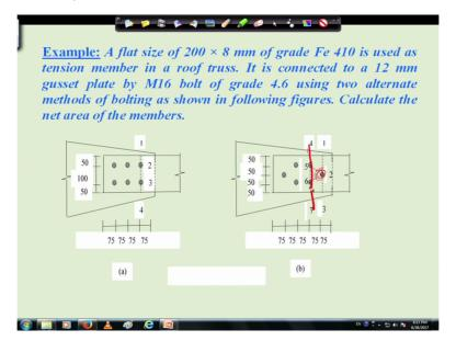
Now another scope is that 4-5-6-7 now 4-5-6-7 means this way now if the plate has to fail along 4-5-6-7 then first it has to fail this due to shear the bolt 2 has to fail, that means when we will be going to calculate the strength along this direction we have to add strength of 2, that means it will be more than the earlier cases therefore we are not going to calculate this because we know it will be more strength will be more so we are not going to calculate.
