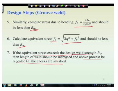
So bending stress also we can find out from this formula that is fb is equal to 6Pe by te into d square, so and depth also has to be less than Rw and then we can find out the equivalent stress equivalent stress will be square root of 3q square plus fb square and that has this equivalent stress has also has to be less than Rw.
