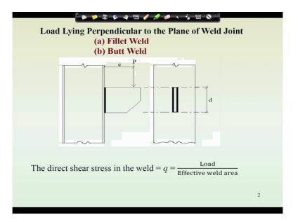
And you know that joint means welded joint means it will be fillet weld and butt weld, the two type of weld joint will be so that we can calculate the stress develop on the fillet weld and stress develop on the butt weld in two cases will come into picture we will discuss two cases.
