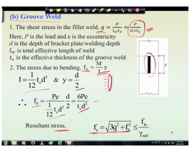
Now the second case is groove weld as I told there are two case one is fillet weld another is groove weld so in case of groove weld you see here the weld has been done by grooving in the plate. So here if we consider the depth of weld as d and thickness as t then we can find out the shear stress and the bending stress in a similar fashion. You see here q is P by lw into te that means here P by d into t not 2d.
