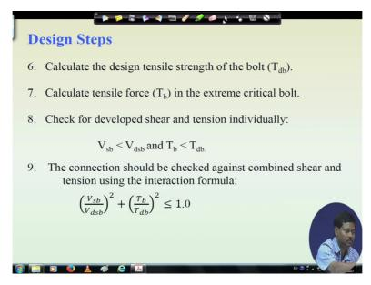
Then in next step what we can find out, we can find out, also the design tensile strength of the bolt group and also the tensile strength in the extreme bolt that also we can calculate and we have to individually check that the force develop on the means shear force develop on a particular bolt should be less than the design shear strength of the bolt and similarly the tensile force develop on the bolt should be less than the tensile strength of the bolt, right.
