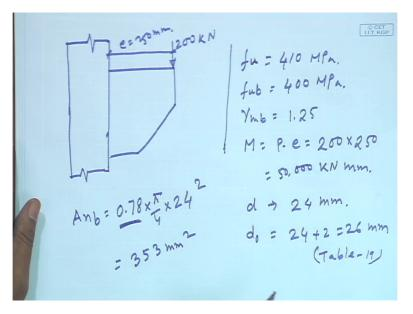
So if I see here that first of all this tension is connected to the bracket and a load of 200 kilonewton which is P at a distance of e is equal to 250 mm these are the two things are given, right. So we have to go for the solution, so here also it has been told that fu that means the grade of steel was fe410 that means the ultimate strength of the steel plate will be fu is equal to 410 MPa.
