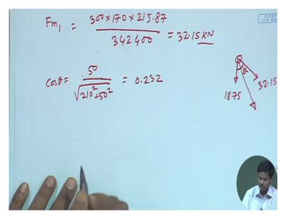
So once we find out now we can find out the value of F2 means Fm right so Fm at number 1 bolt will become 300 into 170 that is M, M into r r is 215.87 Mr by summation r square, summation r square will be 342400. So this is becoming 32.15 kilonewton so in number 1 bolt one load is coming of 18.75 kilonewton and another load due to moment is coming 32.15 kilonewton.
