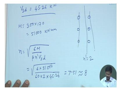
So Vsd value that means strength of bolt design strength of bolt Vsd will become lesser of these two Vdsb and Vdpb that is 45.26 and 78.23 so lesser of these will be be 45.26 kilonewton. So this is the value we got. Now we have now we have to design so we have to decide the number of bolt line so maybe we can start with two bolt line we can start, so if we do so then accordingly we can find out the value.
