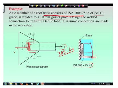
This is the example we have consider today that is A tie member of a roof truss consists of ISA 100 by 75 by 8 angle section of Fe410 grade, is welded to a 10 mm thickness gusset plate that means this gusset plate thickness is 10 mm. Design the weld connection to transmit a load T. Assume connections are made in workshop, right.
