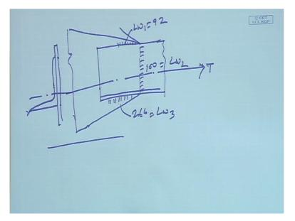
So if we see the angle section if it is connected to a gusset plate, then the distribution this is Lw1, this is Lw2 which is 100 and this is Lw3 so we have to give the value of Lw1 here that is 92 this is 100 and this is 266 mm right.
