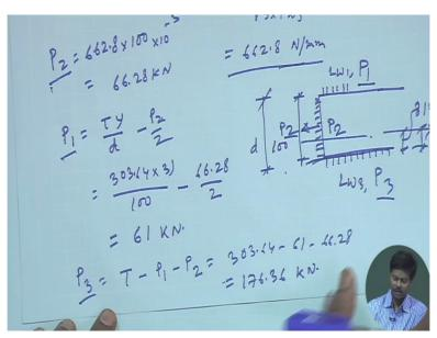
So force to resist at lower site of the angle P3 will be total force minus P1 minus P2 so P3 we can find out that will be 303.64 minus 61 minus 66.28 is equal to 176.36 kilo newton right.
