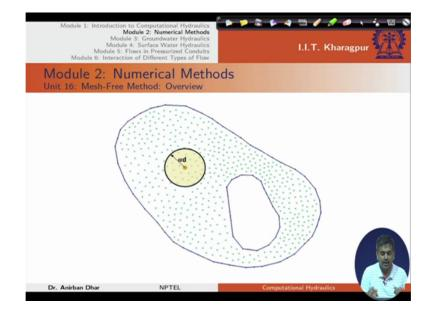
In mesh free method we have seen that polynomial interpolation method is equivalent to our finite difference method if we use NS equals to 3. If we increase the number of points in a particular domain obviously we need to consider more number of points and we will not get that Banded structure like finite difference case.
