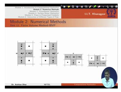
Finite volume method, this conservation laws we have discussed. If there is change in the values in the (down) up gradient and down gradient directions of the cell P then what will be the procedure for numerical flux calculation?
