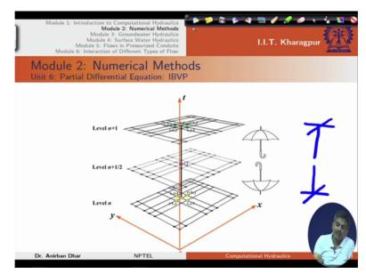
Unit 7 we have discussed this partial differential equation and numerical stability of initial boundary value problem using Von Neumann stability analysis and we have also considered this discretization error, round off error during this stability analysis.
