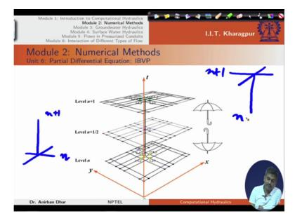
We have also discussed this Crank Nicolson scheme which considers n plus half level which is the intermediate level. And intermediate level we have used half step as explicit and half step as implicit to get the solution.
