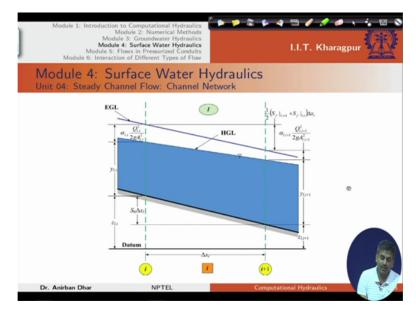
Unit 5 considers the steady channel flow and channel network without reverse flow. If we know the flow direction like this we can directly solve our problem by specifying the flow direction here.
