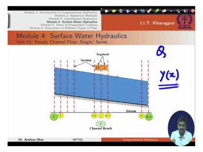
In steady channel flow we have utilized this Q and y as functions because in that case there will be changed in the Q values, different channels in the network.
