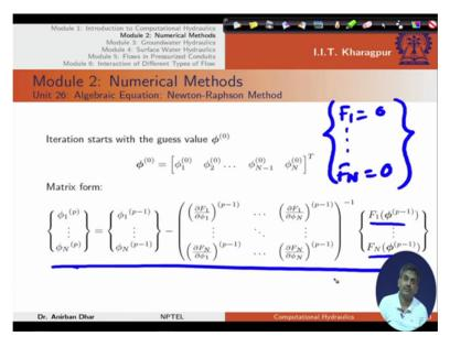
Now in module 3 onwards we have started using scilab as a tool for writing small source code for different kind of problems. So in unit 1 we have utilized scilab for writing this code for one dimensional flow. In one dimensional flow we have utilized this Gauss elimination, our tri diagonal matrix structure for solution of the problem.
