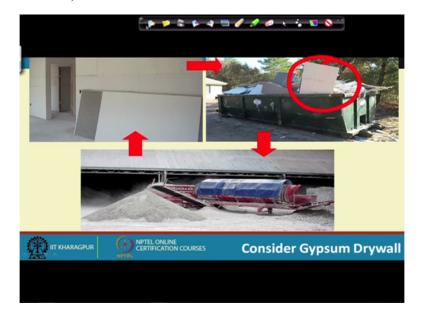
So gypsum drywall essential in the middle is calcium sulphate with 2 molecules of water and then it has a layer of paper on this side, so in the middle we have that and both of my hand is kind of layer of paper where the paper as on that gypsum board. So that is so paper acts as a organic like a paper is the organic present there. So but it is recycle used in a many times in in terms of recycling specially depending on what kind of application they will try to take this paper out.
