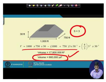
So now using those information if we can do this calculation again here we had 1000 feet length, 750 feet width and 30 feet long with the s of 3, with a slope of 3 we get sorry with a slope of 3, what we are getting here? Is if we can plug the those numbers in here we get volume as 660000 yard cube.
