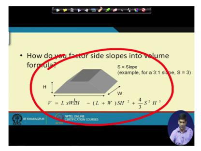
So how do you factor side slope into volume? So this is how the typical volume, I initially when I told you that LWL times W times H that is the very simple way of just doing a rough estimate, but we are when you are doing the actual problem this is what we will do. This is the actual so when we are trying to do the actual problem this is what we need to do. Where this is the this is how the landfill looks like this what you see on this picture and then you have the length, you have the width.
