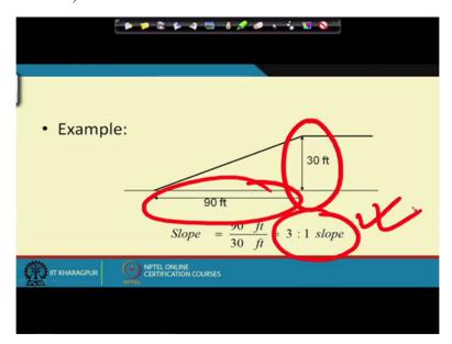
So here as you can see, you have 30 feet so we have 30 feet here so this would be 90 feet in the horizontal, so it is a 3 is to 1 slope and 3 is to 1 slope is what you will see the most common. Say in the exam problem any exam taking where the side slope is not given for the landfill you can take 3 is to 1 as the side slope, because that is the most common side slope used in landfill industry throughout the world.
