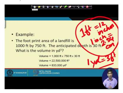
So that is and so based on, say if the footprint of the area of the landfill is 1000 feet by 750 feet, so you have 1000 feet length, 750 feet is your width, anticipated depth is 30 feet, what would be the volume in yard cube? So we can always convert that to meter as well so that is your job as your assignment for you to convert this from feet to meters. I could have done that but I wanted you to do it.
