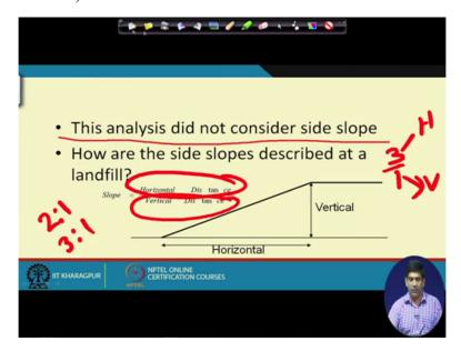
So we got the volume, now how we can use this volume? We can use this volume by so here we are not considering the side slope but in the actual condition when you will be doing the volume calculation you will have the side slope, isn't it? We talked about the landfill has a side slope. So the analysis that we did in the previous slide, we did not calculate the side slope, this analysis did not consider side slope, but actually the side slope will be there at the landfill.
