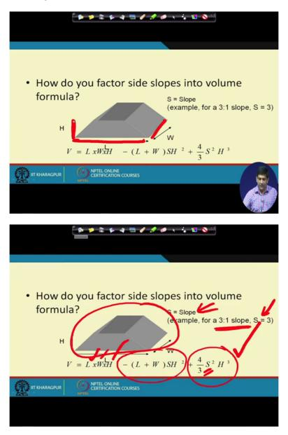
So we have the length of the landfill, we have the width of the landfill, we have the height of the landfill, so we take all these 3 and based on. So this L times W times H that would be if
