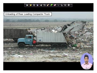
Similarly here unloading of a compactor truck, remember these trucks we looked at it earlier where the waste got collected and it was compacted. Now, we have to take this waste out. So how it is done? Plate which moves along the truck, so that it moves along the truck and then takes this garbage out from the truck. So that is how it works, all these compactor trucks. So we will continue this discussion in our next module. And I will show you some more pictures of this collection.
