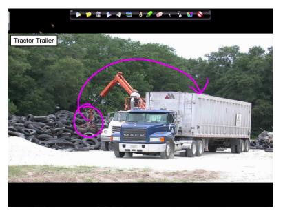
So now we are moving from stationary container to the hauled container system. This is a tractor trailer, here again you lift things up using this tractor and put it in here. So here as you can see, this has been lifted from there and then it will basically, it will be taken and put it in, into this truck and then it will be taken away for like a treatment or disposal.
