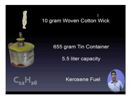
So, it is a 10 graphs of woven cotton wick 655 grams of tin container 5.5 liters of the capacity then the kerosene fuel used for that.
