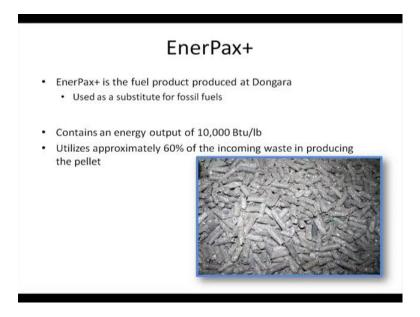
So, it is a fuel product produced in Dongara, you can see the picture over here this is how it looks like the smallest small pallets. And it contains an energy output of around 1000
