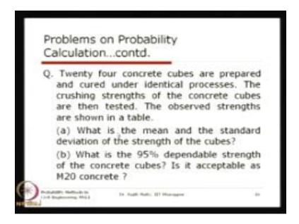
That type of problem is taken as the second problem here that 24 concrete cubes are prepared and cured under the identical process the crushing strengths of the concrete cube are then tested, the observed strength are shown in a table. The question is, what the mean is and standard deviation of the strength of the cube and what is the 95 percent dependable strength of the concrete cubes. Is it acceptable as M20 grade concrete.
