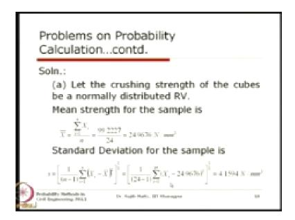
First we are calculating their mean and their standard deviation. So, first the mean is that 24.96, you know that will  $\sum$  divided by 24 is giving that 24.9676 Newton per millimeter square. And second one is that the standard deviation, the sample estimate you know, that 1 by n - 1 x i - x bar square from i = to 1 to n, here n = to 24.So, using this one we get the standard deviation is = to 4.1594. So, we got this two values.
