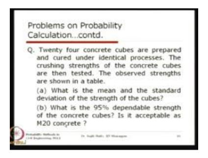
Okay we will go to the next problem, where also the similar the normal distribution is used and this problem is on the testing that strength of concrete and you know that the characteristics strength of the concrete is determined based on this 95 percent dependability.
