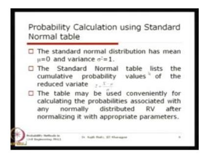
So the standard normal table lists the cumulative probability values of the reduced variate  $z = x - \mu/\sigma$ . So this is important that when so if this x is following a normal distribution which is having the parameter mean  $\mu$  and variance  $\sigma^2$  now you we have also seen in this last module also in the function of random variable you can refer to that this is a 1to1 transformation and this is a linear transformation as well.
