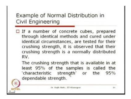
So this is how we define that characteristics strength of the concrete cube.
