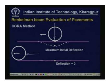
On the other hand, in CGRA procedure initially the load is directly above the point at which we are trying to measure the deflection so the probe point will be here so the dial gauge reading
