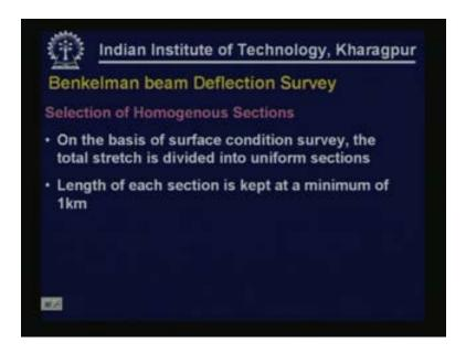
So we can classify the road in terms of cracking, rutting and select homogenous sections on this basis.
