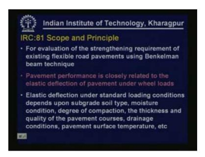
The scope of these guidelines: these are meant for evaluation of the strengthening requirement of existing flexible road pavements using Benkelman beam technique. So this is meant for flexible road pavements and is also meant for Benkelman beam pavement evaluation technique.
