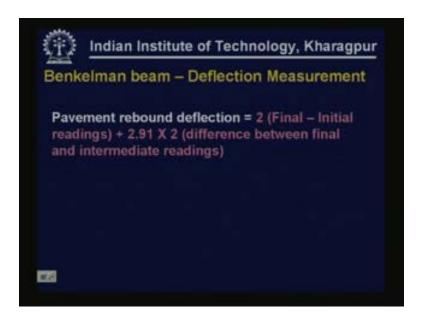
Pavement rebound deflection is twice this is when the intermediate and final readings differ by more than 0.025 mm. Pavement rebound deflection is given as twice final minus intermediate readings plus 2.91 times twice the difference between final and intermediate readings. This is when the intermediate and final readings differ from each other by more than 0.025 mm. If the difference is less the pavement rebound deflection is equal to twice final minus initial reading.
