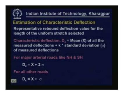
On the basis of number of deflections that we measure in a given stretch representative of a rebound deflection value for the length of the uniform stretch can be selected. This is known as characteristic deflection which represents the overall condition of the pavement. This is obtained Dc is obtained as mean of all the measured deflections plus some factor multiplied by the standard deviation of all the measured deflections.
