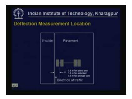
This sketch here shows how to select the location of the points for measuring the deflections. From the pavement edge it is 0.6 m, 0.9 m, 1.5 m for different types of facilities.
