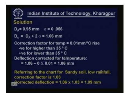
The corrective deflection works out to be 1.06, this is corrected for temperature there is no correction and this is corrected for moisture or season which is 1.03 which is the correction factor so the corrected deflection is 1.09.
