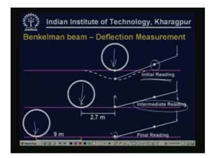
With three positions of the wheel load and the corresponding measurements that we take are represented here. In the topmost sketch we have here the wheel load is directly placed over the point and the probe point is at the bottom of the deflected wall, it is rotating about this hinge and this is the position of the end of the beam for this loading position so we get the initial reading.
