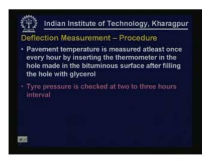
While carrying out the deflection survey we also have to measure the pavement temperature at least once every one hour by inserting the thermometer in the hole made in a bituminous surface and after filling the hole with glycerol. Hence we have to measure the pavement temperature at one hour interval. Tire pressure is also checked at two to three hours intervals and if it is not 5.6 kg per centimeter square we will have to adjust them.
