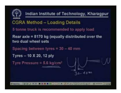
The loading that has to be applied is we have to use a 5 ton truck this is a standard truck so this is to be used to apply the load. What is important is the rear axle of the truck has to weigh 8170 kg. If you recollect this is the load that corresponds to standard axle load 18000 pounds or approximately equal to 80 kilo Newton rear axle.
