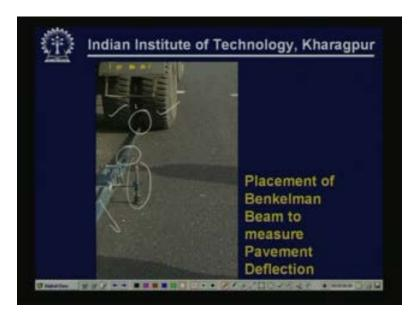
A photograph here shows the dual wheel set of the outer wheel with the probe point of the beam is inserted between the two dual wheels. You may not able to see it very clearly because it is on
