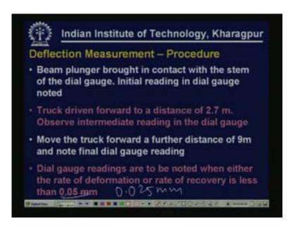
The beam plunger has to be brought in contact with the stem of the dial gauge. Beam plunger is the arrangement that we have at the end of the beam above which the plunger of the dial gauge will be resting. So as the beam rotates in this direction the plunger of the beam will be supporting the plunger of the dial gauge.
