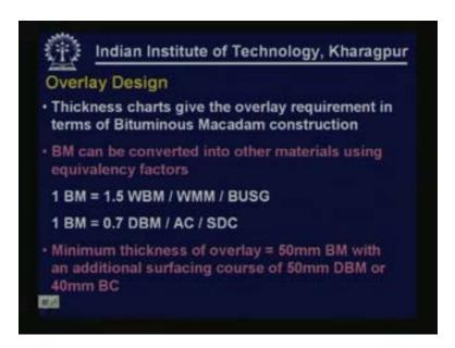
We may not be using bituminous macadam. obviously bituminous macadam cannot be used for surface so this has to be replaced by the total beam requirement that has to provided in terms of DBM, also it can be BM, BM, BBM, BC or other types of bituminous layers. So using the conversion factors that are given here we can convert the total requirement of BM into different component layers.
