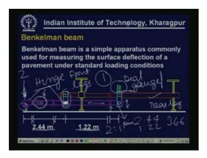
Benkelman beam is a very simple apparatus and it is commonly used for measuring the surface deflection of a pavement under standard loading conditions. A schematic arrangement of the Benkelman beam is shown here. This is the Benkelman beam (Refer Slide Time: 11:11). It is cut at several places because its full length cannot be shown in sketch. This is the probe point which would be resting on a pavement surface at a point at which we are trying to measure the deflection.
