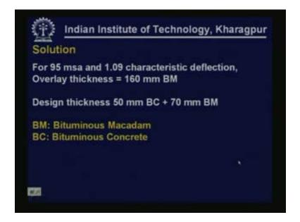
So for 95 million standard axles and 1.09 characteristic deflection using the thickness charts given in IRC the total overlay thickness works out to be 160 mm of bituminous macadam. So I split this into 50 mm of BC and 70 mm of BM. So you can verify whether this is correct or not. BM is bituminous macadam and BC is bituminous concrete.
