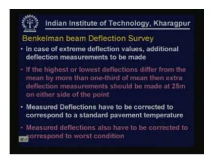
In case of extreme deflection values the additional deflection measurements are to be made. For example, if the highest or lowest deflection differs from the mean by more than one third of the mean then extra deflection measurements should be made at 25 m on the either side of the pavement. We have to be careful about extreme points or extreme deflections then we have to make additional deflections if this criteria is satisfied.
