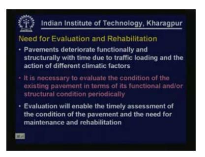
We have briefly discussed about the need for evaluating pavements in the previous lesson 5.1. We know that once constructed pavements gradually deteriorate in terms of its functionality and also in terms of its structural condition. The structural strength also gets reduced, there will be cracks, there will be deformation, there will be deterioration of materials in various forms resulting into reduced structural soundness of the structure.
