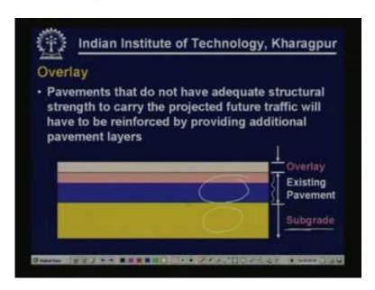
Overlay is that reinforcing layer that we provide over an existing pavement. That is because pavements that do not have adequate structural strength to carry the projected future traffic will have to be reinforced by providing additional pavement layer.
