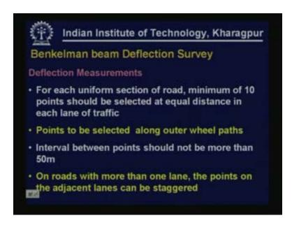
For each homogenous or uniform section of road a minimum of ten points should be selected at equal distance in each lane of traffic.
