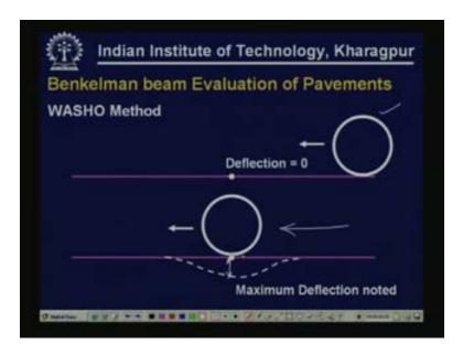
The WASHO method of measuring deflection using a Benkelman beam is depicted here. In this case initially the load is away, the probe point of the beam is kept here so we measure the corresponding deflection, so as the wheel load gradually moves forward and is directly above the point that is when we are expected to get the maximum deflection so we closely monitor the reading in the dial gauge. So when it is directly above the point that is the deflection we note in the case of a WASHO procedure.
