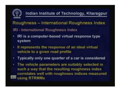
IRI is a computer-based virtual response type system. This is not something that we are going to measure. We cannot measure IRI but we can compute from some given inputs. So whatever value we measure it's a standard value. There are no physical practical parameters that are going to influence this parameter this is a theoretically computed value.
