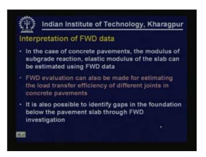
In the case of concrete pavements the modulus of sub-grade reaction, elastic modulus value of slab can also be estimated, FWD evaluation can be used to estimate the load transfer efficiency of joints in the concrete pavements, and it can also be used to identify gaps below the pavement.
