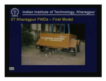
We can see the mass spring system, we can also see the geophones placed behind the trailer to measure the deflections.
