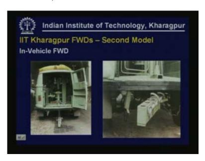
You can see the details of the falling weight deflectometer here. What you see on the right hand side and the left hand side is the extendable foldable geophone placing arrangement.
