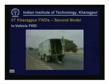
National highway 6 is being evaluated using the falling weight deflectometer in-vehicle.
