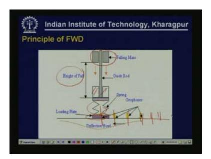
This sketch here explains the principle of a Falling Deflectometer. As you can see there is a falling mass raised to certain height and there is a loading plate here and there is a spring arrangement so the mass is made to fall on the spring which in turn transmits the load to the
