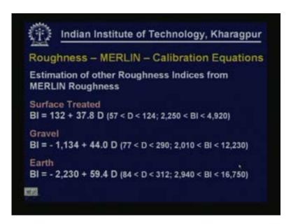
Similarly for surfaces that are treated the BI can be estimated from MERLIN using this equation, for gravel, for earth surface also different correlations are available as you can see here. We should also note the range of D values and the range of BI values for which these equations are applicable.
