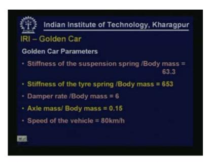
These are the golden car parameters that are used. stiffness of the suspension system by body mass is taken as 63.3, stiffness of the tire spring by body mass is taken as 653, the damper rate by body mass is taken as 6, axle mass by body mass is taken as 0.15 and the speed at which the vehicle is made to move in the theoretical model is 80 km per hour.
