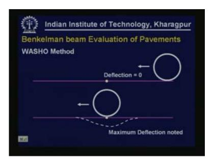
The WASHO procedure is depicted here. In the WASHO procedure initially the load is away from the point so deflection is 0 and as it approaches and is right over the point we observe the maximum deflection.
