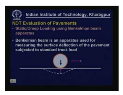
The other most commonly used method is the Benkelman beam apparatus. This can be done either in static load or creep loading condition. We will not go into the complete details about the Benkelman beam procedure because we will be covering this in the next lesson when we talk about design of overlays using Benkelman beam apparatus.
