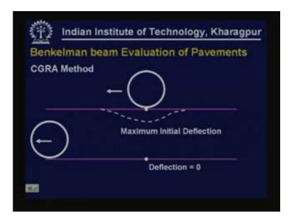
In the other procedure CGRA initially the load is on the point itself so you already have the maximum initial deflection so when you remove the load away from the point deflection theoretically has to become 0 then the difference is the rebound deflection.
