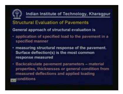
The general approach of a structural evaluation method will be to apply a specified load to the pavement in a specified manner. The load applied and the manner in which it is applied has to correspond to the theoretical model that we are using or the model that we are using in making interpretations about the pavement condition.
