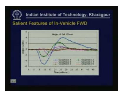
This diagram show shows a typical output obtained from the geophones. Each one of these lines represents different deflections measured in different locations.
