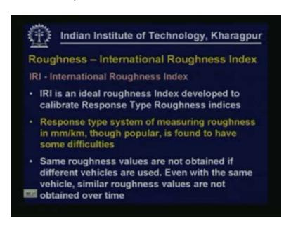
The next and most commonly used roughness index worldwide is the international roughness index. This is a very interesting concept in terms of expressing roughness of a given road. IRI is the International Roughness Index. This is an ideal roughness index developed to calibrate response type roughness indices. Basically IRI concept has been evolved to calibrate various
