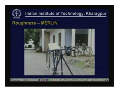
This is a photograph of a MERLIN machine. As you can see this is a very simple apparatus. You can see the front wheel, you can see the rear leg, you can also see the counter weight here, this is the hinge part, you can see the counter here though it may not be very clear and this is the moving arm.
