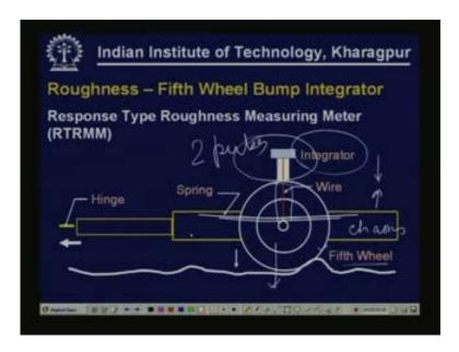
The roughness in terms of bump integrator value is normally measured using equipment called as fifth wheel bump integrator. This comes under the class of roughness meters known as response type roughness measuring meters. The roughness of the road can be obtained in terms of the surface profile.
