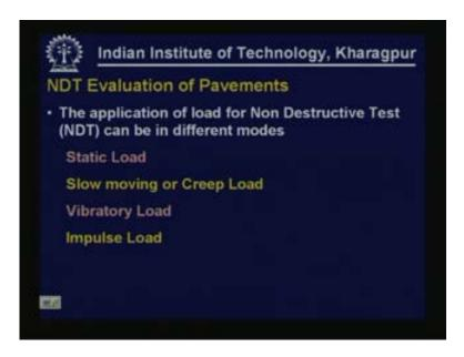
The application of load for NDT testing can be done in different modes. It can be a static load, it can be slow moving or creep load it can be vibratory load, it can be impulse road.
