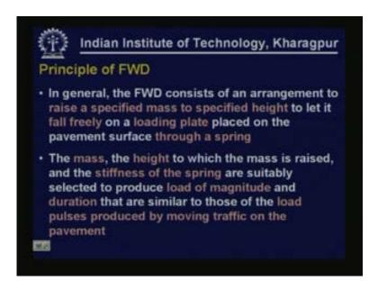
In general FWD consists of an arrangement to raise a specified mass to specified height and to let it fall freely on a loading plate placed on the pavement surface through a spring. The mass, the height to which the mass is raised and the stiffness of the spring are suitably selected to produce a load of magnitude and duration that are similar to those of the load pulses produced by moving traffic on the pavement.
