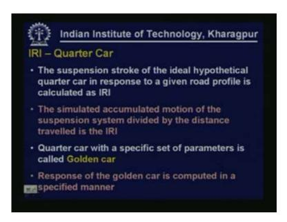
The suspension stroke of the ideal hypothetical quarter car in response to a given road profile as it is made to move over a road having different characteristics so the quarter car response the suspension system of the quarter car response the suspension stroke is calculated as IRI.
