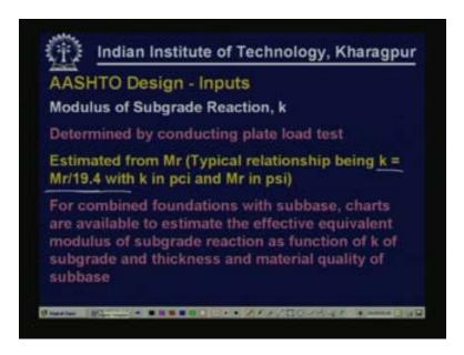
The modulus of subgrade reaction k has to be determined by conducting a plate load test. It can also be estimated from the resilient modulus value of a subgrade material if the resilient modulus value is available. It can be obtained as k = Mr by 19.4 where k is in pci and Mr is in psi.
