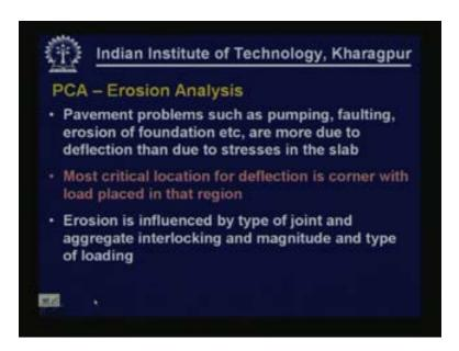
Coming to erosion analysis that is considered in PCA analysis pavement problems such as pumping, faulting and erosion of foundation etc are more due to the deflection than due to stresses in the slab. Deflection is the consideration that we have to be concerned about. If there are more deflections there is going to be more amount of pumping, more amount of erosion and more faulting problems also are likely to be there if the slab deflects more.
