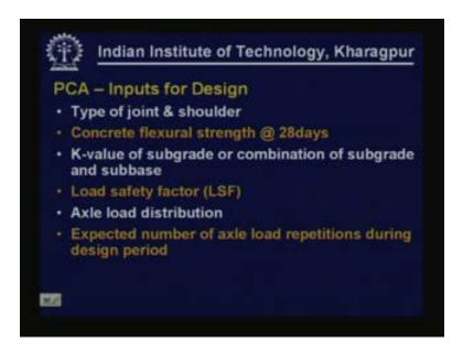
The other inputs that are required for design are what type of joints are provided, what is the type of shoulder that is there; concrete shoulder, unpaved, tight concrete shoulder etc, so different PCA gives design provisions for different types of shoulders.
