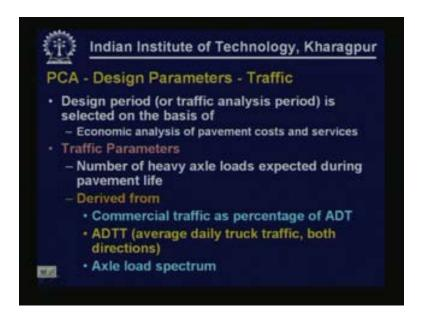
Other design parameters relating to traffic are; we have to select a design period or the traffic analysis period, this has to be selected on the basis of economic analysis of pavement costs and services. Other traffic parameters are selecting number of heavy axle loads expected during the pavement life. These are to be derived from commercial traffic as percentage of average daily
