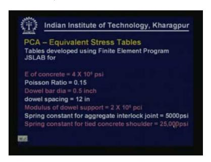
These stress analysis tables were developed using a finite element program JSLAB for the following data:
