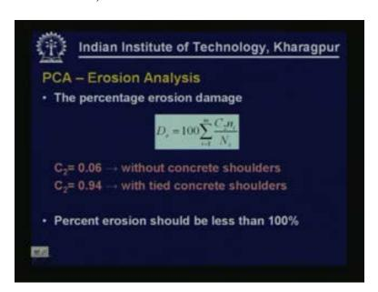
Percentage erosion damage, again here we are going to have different magnitudes of loads and different magnitudes of load would produce different amount of deflection so the erosion damage caused by different axle load groups will be different so we have to sum up all the damage caused because of all the groups of axle loads so this is how we do the summation. So the total erosion damage is again a summation of a multiplication factor C2 small ni divided by capital Ni
