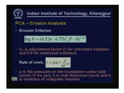
This is the erosion criteria that PCA adopts to estimate how many repetitions the pavement can sustain before unacceptable levels of erosion takes place before the slab or the foundation fails because of erosion failure. This is given as  $\log N = 14.524 - 6.77$  into C1 P – 9 to the power 0.103. In this case C1 is an adjustment factor. To account for different types of sub-bases that are used C1 will be one for untreated granular sub-base and C1 will be 0.9 for stabilized sub-base.
