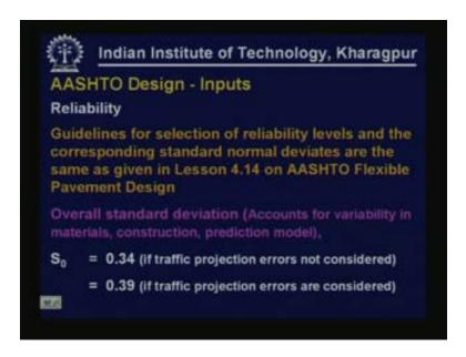
Reliability: Obviously for different types of facilities we go for different levels of reliability. The overall standard deviation which accounts for variability in materials, variability in construction, variability in prediction models can be selected as 0.34 if traffic projection errors are not considered and 0.39 if traffic projections errors are considered.
