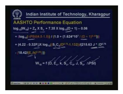
This is the performance equation which is the heart of design of concrete pavements using AASHTO procedure. As you can see here the number of repetitions which is expressed in terms of standard axle load repetitions is expressed as a function of all the pavement parameters and the reliability parameters.
