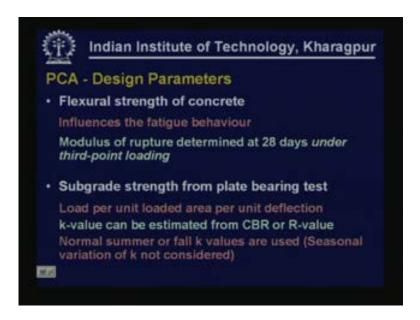
The flexural strength of concrete influences the fatigue behavior of concrete.
