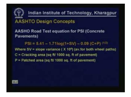
So the AASHO road test equation for present serviceability index for concrete pavements is given as present serviceability index is equal to  $5.41 - 1.71 \log 1 + SV - 0.09$  multiplied by C + P under root. We discussed about slope variance in the lesson on design of flexible pavements as per AASHTO procedure.
