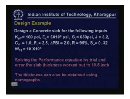
Here is the design example. You have to design a concrete slab for the following inputs:
