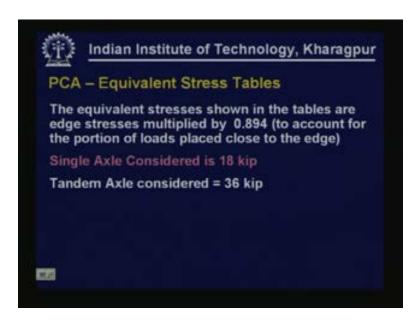
The equivalent stresses shown in the tables are edge stresses multiplied by 0.894. This is to account for the portion of loads placed close to the edge. So it's assumed we are considering only those loads which are going to be placed close to the edge so to account for that the stresses are already multiplied by a factor of 0.894.
