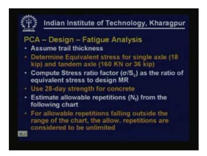
The fatigue analysis proceeds like this; we assume a trial thickness and determine equivalent stress for single axle that is 18 kip axle and tandem axle that is 36 kip axle. We determine these from the tables for a given slab thickness for a given k-value and for either single axle or tandem axle as you have seen in the previous slide we have equivalent stress values available for both single and tandem axle so we can select those values from those tables.
