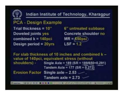
Starting with a trial thickness of about 10 inches for the 6 inches untreated sub-base that we have provided let us assume we are going to provide dowel joints there is no concrete shoulder so the combined k-value is selected from the charts that are available from PCA as 140 pci, MR is given as 650 and this being an important road we will select a load safety factor of 1.2, the design period let us consider to be 20 years.
