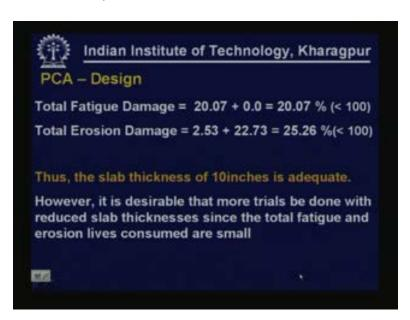
So the total fatigue damage caused by single axle load groups and tandem axle load groups is 20.07 + 0 that is a total of 20.07 which is of course well below 100% and the total erosion damage is 2.53 + 22.73 = 25.26 which also is well below 100%. So obviously the thickness that was selected is quite safe. However, it is desirable that more trials be made to reduce the slab thickness because the slab is over safe in this case.
