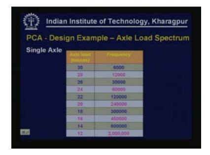
For single axle for different load groups this is the frequency. For example, for the load group having a midpoint value of axle load of 30 tons there are going to be about 6000 repetitions. Similarly for a load group having a midpoint of 16 tons we are going to have about 450,000 repetitions. Similarly axle load spectrum for tandem axles is also given in the slide.
