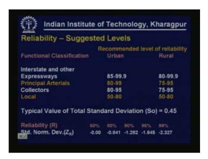
Normal reliability levels that are suggested are; depending on the type of pavement different levels of reliability are suggested. Obviously for express ways high levels are reliability, for local roads low levels are reliability. The standard normal deviates that are used for different levels of reliability are; for 99% it is -2.327, for 95% it is -1.645 so these are standard values depending on normal distribution.
