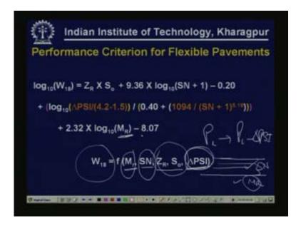
This is the performance criteria used in AASHTO flexible pavement design.
