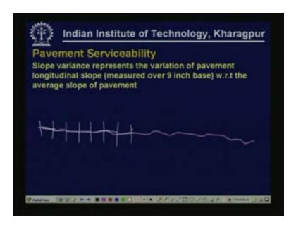
A slope variance represents the variations of pavement's longitudinal slope this is measured over 9 inch base as I have just explained in the previous slides. Thus in the 9 inch base length is considered and over this is where the slope is measured. So, if you have hundred such n values you can calculate the variance of all those n values.
