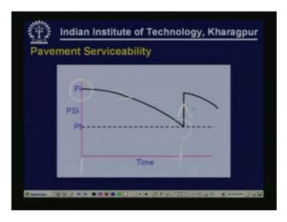
As we have indicated earlier the performance of the pavement can be represented by the serviceability index of the pavement. For example, in this chart we see the present serviceability index is going to vary with time. So soon after construction this is the serviceability index that is available but with time this is going to deteriorate. In what manner it is going to deteriorate or
