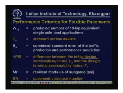
Similarly the other parameters that are used in the performance equation is Mr which is the resilient modulus value of the subgrade and the structural number SN which is the pavement structural number.
