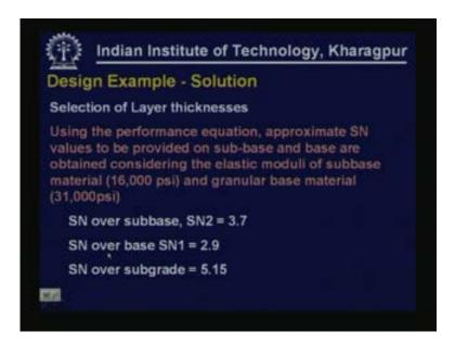
So the structural number corresponding to each individual layer can also be selected by using the appropriate modulus values for each layer. We have already done the subgrade and the structural number required is 5.15. By selecting the modulus value for subbase putting that in the equation you can get the structural number required that is 3.7. Similarly by putting the modulus value of granular base in the equation you can get the structural number of 2.9 as indicated here.
