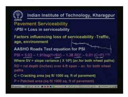
The area of cracking is expressed in terms of square feet for thousand square feet of paved area. If you observe thousand square feet of paved area out of that how many square feet has got cracked surface that is what is known as cracked area. Similarly patching is defined by how much area of the paved surface is patched per thousand square feet of pavement area.
