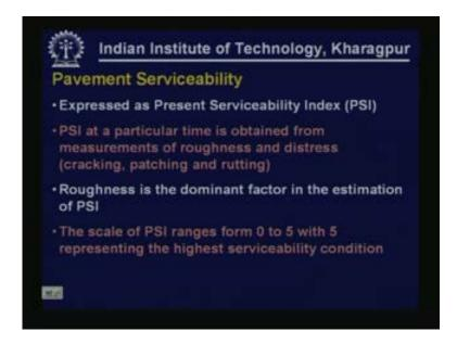
Roughness is the dominant factor in the estimation of PSI. If you see the expressions available for estimating PSI as a function of various physical parameters main parameters that are available are roughness, cracking, patching and extent of rutting. Roughness is the dominant factor in the estimation of PSI. The scale of PSI ranges from 0 to 5 with 5 representing the highest serviceability condition obviously 0 represents the worst condition that is possible.
