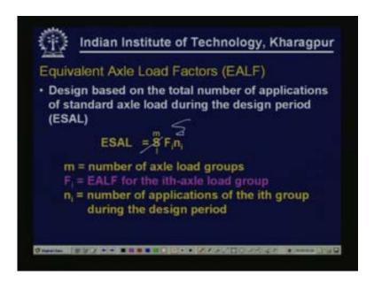
So the total number of equivalent standard axle load repetitions can be obtained using this expression (Refer Slide Time: 29:56). In fact the design based on the total number of
