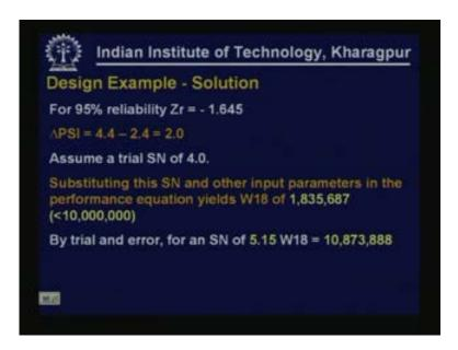
For 95% reliability  $Z_R$  value is 1.645, delta PSI is 4.4 - 2.4 = 2. Assuming a trail structural number of 4 substituting this in the performance equation  $W_{18}$  left hand side works out to be
