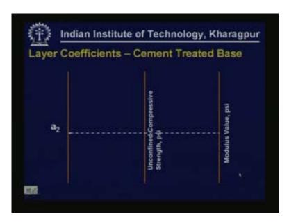
Similarly layer coefficients estimation can be done on the basis of unconfined compressive strength or the modulus value of cement treated base.
