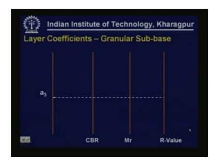
This nomograph indicates how one can estimate layer coefficient for granular surface again on the basis of CBR, Mr and R value.
