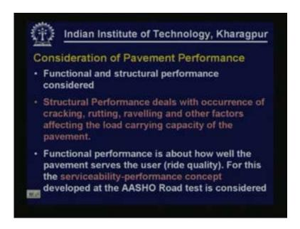
The functional performance is about how well the pavement serves the user especially the right quality. For this the serviceability performance concept is used; how well the pavement is able to serve, what is the level of serviceability available at a given point of time and so on is the concept is used in AASHO guidelines for describing the performance of the pavements. In fact this was the concept that was developed during the AASHO road test.
