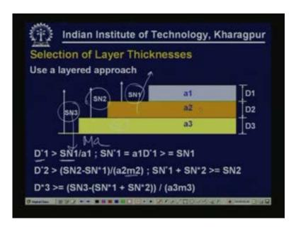
We can use the layered approach to determine what should be the thickness of each individual layer. What is shown here is if you can estimate the structural number required above subgrade this can be estimated by knowing the Mr value of the subgrade. Similarly if you can assign elastic modulus value to the subbase so putting that value in the equation we can get SN2.
