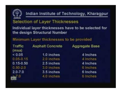
We have to put all these inputs in the performance equation  $W_{18}$  equal to as a function of all the parameters that were given earlier and putting all these parameter there we can work out the structural number from that equation. So what we get is the structural number from that equation and that has to be split into different layer thicknesses and different material properties.
