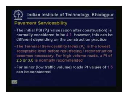
The initial PSI that is Pi this value which is seen or which is measured which can be estimated soon after construction is normally considered to be about 4.2 for flexible pavements. This can be different depending on the type of material that we use, type of construction techniques that
