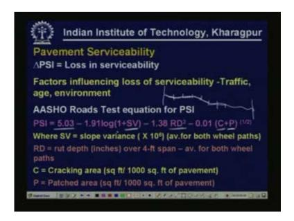
Delta PSI is what we are going to be looking at, this is the loss in serviceability. If we start with an initial serviceability of Pi with time the serviceability is going to be deteriorating. So we are going to be talking about what is the loss in serviceability that is going to be permitted over the design life period.
