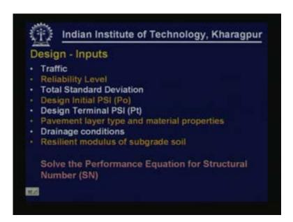
So the design inputs that are used for designing pavements are; we have to have information on traffic, we have to select the reliability level, we have to estimate or take the values from the guidelines about total standard deviation, we also have to select an initial PSI depending on the
