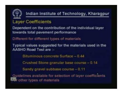
The layer coefficients depend on the contribution of the individual layer towards total pavement performance. They will be different for different types of materials. Typical values suggested for materials used in the AASHO road test in the early 1950s are bituminous concrete 0.44, crushed stone granular base 0.14, sandy gravel subbase course 0.11. There are guidelines available for selection of layer coefficients for other types of materials also.
