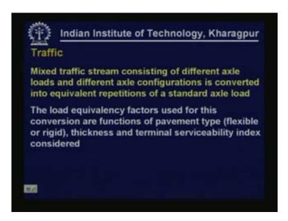
Mixed traffic stream consisting of different axle loads and different axle configurations is converted into equivalent repetitions of a standard axle load because traffic is considered in terms of repetitions of standard axle loads standard axle load being 18,000 pounds 18 kip or 18 kilo Newton load.
