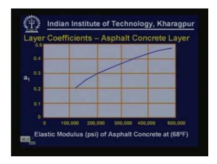
For example, if we are trying to select layer coefficient for the Asphalt concrete layer if you know the modulus value of Asphalt concrete at 68 degrees Fahrenheit temperature we can select
