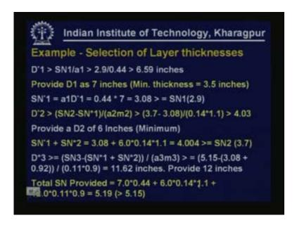
So this is how we can work out individual layer thicknesses as we have explained in the procedure in the previous slide. You can see the calculations here.
