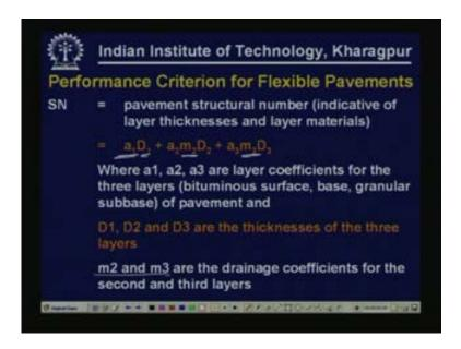
As I mentioned earlier SN is a single index that indicates the strength of the pavement. We know pavement consists of number of layers and what we are representing as pavement represents all those layers that are above the foundation. There can be three layers or four layers, it can be having different kinds of materials and these materials may be affected by different climatic conditions in a different manner so taking into consideration all those things one single
