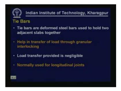
As I just indicated tie bars are deformed steel bars and these are placed to hold the two adjacent slabs together. They indirectly help in the transfer of load through granular interlocking. Load transfer is provided by the tie bars themselves there are also steel bars placed across the joint but the load transfer provided through the tie bars is usually negligible and not generally taken into account. These are normally used for longitudinal joints.
