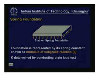
As I said spring foundation is the most common assumption that we make about foundation of concrete pavements. in this the foundation is represented by its spring constant known as modulus of sub-grade reaction k. k is normally determined if this is being determined from a field test it is determined by conducting a plate load test on the foundation.
