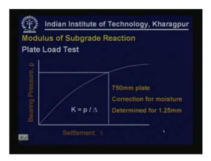
The slope of this diagram at a specified deflection is taken as modulus of sub-grade reaction. normally we use 750 mm dia plate to conduct plate load test and we also have to normally make
