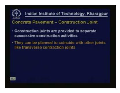
There is another type of joint that is necessary because at the end of construction one cannot construct a hundred kilometer length of slab continuously it has to be stopped and started again so you have construction joints when you stop work and start again.
