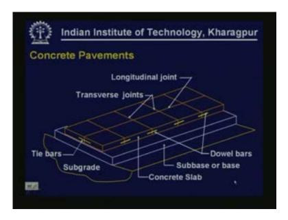
This is the general arrangement of a concrete pavement. right at the bottom you will have the sub-grade above which there will be a sub-base or base that is this layer (Refer Slide Time: 6:37) over which will be placed number of panels of concrete slabs.
