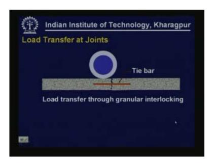
We can also expect load transfer through granular interlocking also if we just provide only tie bars. So this is a situation where we have crack developing through the slab and we have provided tie bars to ensure that the slabs do not get separated, this is one type of load transfer mechanism. Another mechanism is we can also have cracking, granular interlocking, we can also have dowel bars so both granular interlocking and dowel bars together provide this load transfer mechanism.
