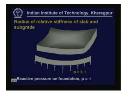
There is a parameter that we normally use to represent the relative stiffness of the slab and the sub-grade. The slab will have one stiffness and the foundation will have different stiffness. To have an index which represents the relative stiffness of slab with reference to the sub-grade we use a term called as radius of relative stiffness. The assumption using which the radius of relative
