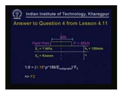
Then granular thickness of known thickness is built over this, plate load test is conducted on a two layer system. so for a rigid plate this is the expression for surface deflection 'p' is known, 'a' is known, surface deflection is also known, E sub-grade is also known so now we can find out  $F_2$  from this plot.
