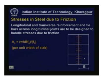
We can provide longitudinal or transverse reinforcement and tie bars across longitudinal joints to handle these stresses. The area of reinforcement to be provided is given by this expression where 'b' is the width of the panel and f s is the allowable stress.
