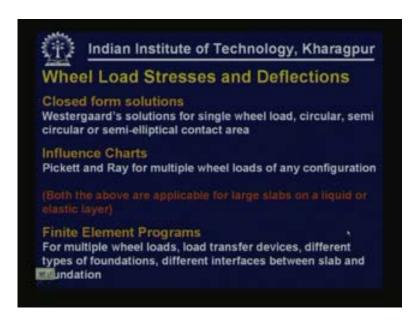
Closed form solutions are available given by Westergaard's for single wheel load, circular contact area or semi-circular contact area or semi-elliptical contact area but circular contact area is the most commonly used shape of load contact.
