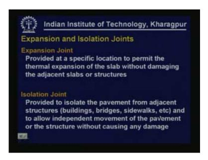
We also have expansion and isolation joints in general they are similar in their function. Expansion joint is provided at specific location to permit thermal expansion of slab without
