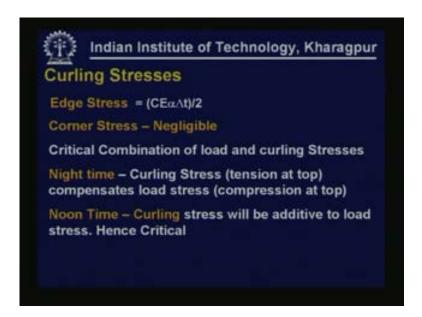
The curling stress in the edge region can be estimated by the expression coefficient multiplied by elastic modulus value and coefficient of thermal expansion temperature gradient by 2. In the corner region the curling stress is normally negligible because the retrain provided by self weight is almost negligible there. The critical combination of load and curling stresses that is to be
