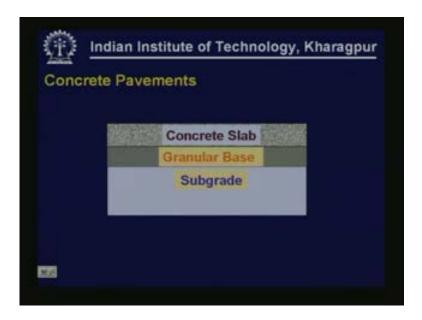
This is how a typical concrete pavement would look like. it will have sub-grade, sub grade though it shown to be of finite thickness it will be of infinite thickness, the top portion as we have learnt earlier will be of prepared foundation prepared to proper specification and strength over which you may have a granular base or sub-base depending on the requirement and over which we have a concrete slab.
