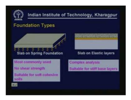
This slide here shows the two types of foundation. On the left hand side you have slab placed on a spring foundation or winkler foundation or dense liquid foundation. This is the most commonly used foundation type for analysis of concrete pavements. It assumes no shear strength for the foundation and these are usually suitable for soft cohesive soils.
