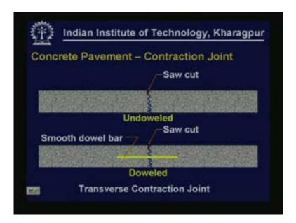
So load transfer will be through this granular interlocking and also through the dowel bar system that is placed. There will be a number of dowel bars placed across the width of the slab so all these dowel bars acting as one system will be transferring load from this slab to the adjacent slab. But load will be transmitted from this slab to the adjacent slab through the granular interlocking mechanism also.
