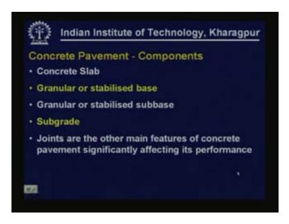
So as we have just seen these are the components that a concrete pavement will have, concrete slab, granular or stabilized base, their base can be either a granular base or it can stabilized base, it can be dry lean concrete base, it can also have a granular sub-base, it can be stabilized sub-base also and it will of course have a sub-grade also. Joints are the other main features of concrete pavement which significantly affect its performance.
