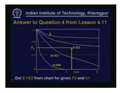
So once we know  $F_2$  from  $F_2$  and from known thickness we can obtain the ratio of E1 by E2. Next we have to find out what is the thickness of the layer to be provided. We know the subgrade modulus value, the allowable deflection is 0.2 this is a flexible plate so 1.5 pa by  $E_{\text{sub-grade}}$  into  $F_2$  so E2 has to be obtained  $E_{\text{sub-grade}}$  is known, 'p' is known, 'a' is known, surface deflection
