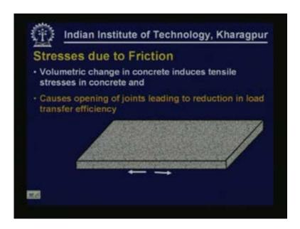
Let us understand why there will be stresses in the slab because of friction. Volumetric change in concrete induces tensile stresses in concrete. We are referring to a case where it is trying to contract. This would also cause opening of joints leading to reduction in load transfer efficiency.
