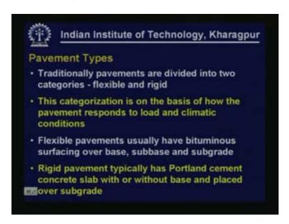
As we have already discussed in earlier lessons traditionally pavements are divided into two categories; flexible and rigid. This categorization is mainly on the basis of how the pavement materials or pavement as a whole responds to load and climatic conditions.
