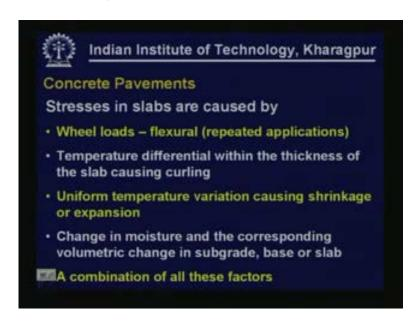
There are going to be stresses produced because of temperature differential within the thickness of the slab. Because if there is temperature differential within the slab that means top temperature is more than bottom temperature or bottom temperature being more than top temperature so slab either curls up or curls down. This also can produce stresses in the slab. We will discuss how to calculate that, what type of stresses is produced and so on.
