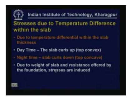
As I indicated earlier there are going to be stresses within the slab due to temperature difference also. Due to temperature differential within the slab during day time the slabs tries to curl up and the top will be convex and during night time the slab curls down and the top will be concave so due to weight of the slab and the resistance offered by the foundation the stresses are going to be induced.
