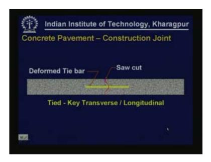
We can have another type of construction joint that is instead of making a butt joint we can make a key joint. As you can see here there is a key arrangement here and these are also complemented by insertion of tie bars if it is a longitudinal joint you can also have it for a transverse joint then you can have dowel bars also placed across these two slabs. But since you are providing a key normally you may not require dowel bars there because through this key load transfer can be ensured.
