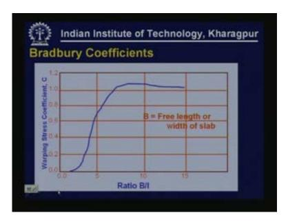
Bradbury has given coefficients to find out what is value of sigma suffix x and sigma suffix y depending on the dimension of the slab with reference to the radius of relative stiffness. If we know the dimension of the slab for example  $1 \times y \cdot 1$  then we can find out what is the corresponding coefficient that is  $C_x$ .
