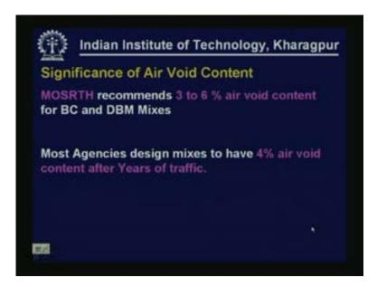
The Ministry of Shipping and Road Transport Highways recommend 3 to 6% air void content for bituminous concrete mixes and DBM mixes. But most agencies design mixes to have an air void content of 4% after years of traffic. What we have to remember is we are targeting at air void content which would be obtained after years of traffic.
