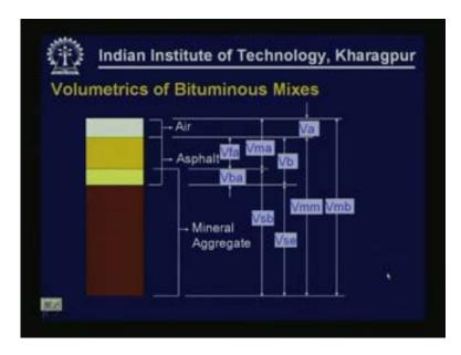
This is again represented in this schematic arrangement. We have volume of mineral aggregate, part of this has been filled with bitumen assuming that there are surface voids which can be filled
