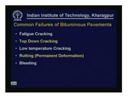
As we have seen in the previous slides there are various types of failures; fatigue cracking is a cracking that is caused by repetition of load or thermal stresses, top down cracking, low temperature cracking and so on. Cracking can also be because of very low temperatures, mix trying to shrink and the restrain that is provided to the mix from being shrunk can cause low
