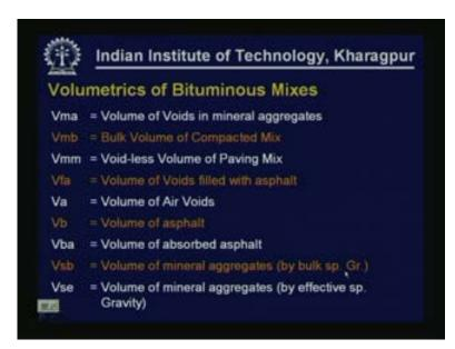
Various terms that we have used in the previous slide are Vma: this is the volume of voids in the mineral aggregate, Vmb: this is the bulk volume of the compacted mix. Obviously we are going to use aggregates we are going to use binder put them together, heat them and then compact them using certain compaction effort so what you finally get is a compacted mix and within that mix there will be some air voids so we are referring to the volumetrics of the compacted mix.
