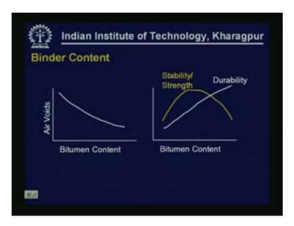
Now the most important task that is to be done is you have to select and aggregate skeleton structure, then you have to select an appropriate binder content to be used, optimum binder content. What happens when you go on increasing the bitumen content for a given aggregate gradation structure? Obviously the air void content is going to get decreased. And when you gone increasing the bitumen content this stability increases up to a certain point then it starts decreasing.
