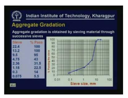
Normally this is how we represent the gradations in a graphical form. The x axis would be sieve size on a log scale and y axis will be the percentage passing through the given sieve which will be on a normal scale.
