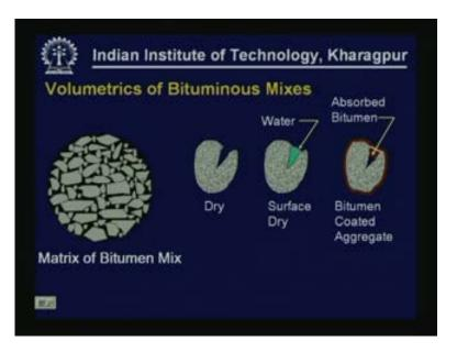
To convert a given quantity of bitumen say 100g of bituminous mix into volumes of the corresponding constituents that is volume of aggregate, volume of binder and obviously there is also going to be some air void content so to calculate those air void contents we need to have the specific gravity of all these components. If you know the weights and also if you know the specific gravities we can of course calculate the volume of each component and then express in terms of percentages.
