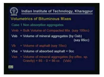
Let us consider two different cases and see how the volumetric is different. Case one is we are considering aggregates that are non absorptive. There are no surface pores so neither water nor bitumen can penetrate into the surface pores, let's consider that case. Let us consider the bulk volume of the compacted mix let us say 100 cc represented by Vmb. Let us consider the volume of mineral aggregates that has been used in the mix.
