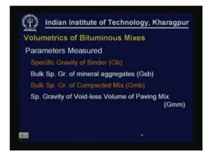
To calculate all these volumetrics the parameters that we need to measure will be specific gravity of binder, bulk specific gravity of mineral aggregate, bulk specific gravity of compacted mix, specific gravity of void less volume of paving mix that is Gmm.
