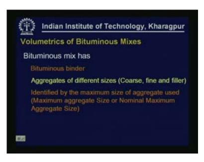
Bituminous mix usually is designed in terms of its volumetrics. We will discuss later why we design in terms of volumetrics. Bituminous binder has got aggregates of different sizes, coarse, fine and filler. The aggregates are identified in terms of the maximum size of aggregate which in turn can be represented in terms of maximum aggregate size or nominal maximum aggregate size.
