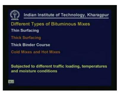
As I indicated these are thin surfaces. There are also thick surfaces. We would consider some of those surfaces whose thickness would be 20 mm, 25 mm to be thin and surfaces having 40, 50 mm thickness as thicker surfaces, we can have thick binder courses and the mixes can be cold mixes as well as hot mixes.
