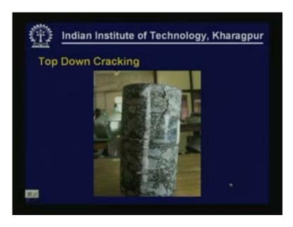
But we can also have cracks that initiate from top and progress downwards as can be seen in the core of bituminous pavement that has been taken out. You can see the crack that is initiated from the top and progressing to the bottom. These are what are known as top down cracks caused by various reasons and various conditions. These also need to be taken into consideration while designing the mixes.
