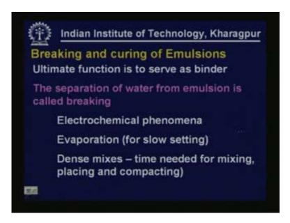
As we said ultimately we need bitumen to be left behind and water should go away. So the removal of water from emulsion is called as breaking. Breaking is a process which occurs through various phenomena. It could be electrochemical phenomena; it can be through evaporations especially for slow setting emulsion. For dense mixes the time needed for mixing, placing and compaction will also have to be assessed.
