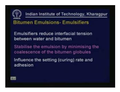
The emulsifiers reduce the interfacial tension between water and bitumen and they stabilize the emulsion by minimizing the coalescence of bitumen globules, this is what we discussed in the previous slide and the emulsifiers that we select influence the setting or also known as curing rate and adhesion.
