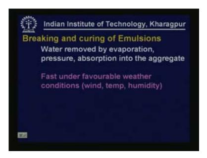
The water is normally removed by evaporation; it can be by mechanical means application of pressure, absorption into the aggregate. It normally happens faster under favorable weather conditions such as the condition that we referred to would be wind, temperature and humidity.
