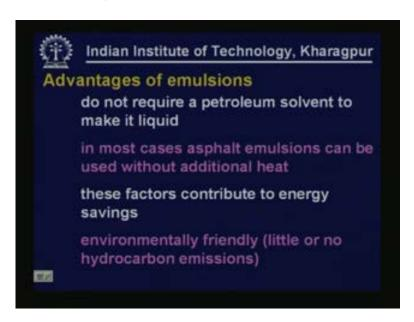
The main advantage of emulsions is, they do not require petroleum solvent to make it liquid. This is in comparison to cutbacks. In most cases asphalt emulsions can be used without additional heat. These factors contribute to energy saving because we don't have to use heat so we can save energy.
