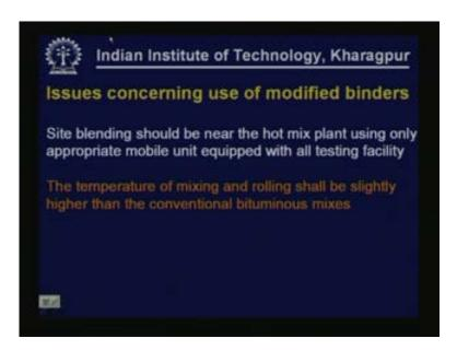
Site blending: in many cases the blending of rubber with bitumen, blending of polymer with bitumen is permitted but this should be done close to the hot mix plant by only using appropriate mobile unit. The temperature of mixing and rolling shall be slightly higher compared to conventional bitumens. When we are using modified bitumens all the temperatures normally related to mixing, rolling and other things will be slightly higher compared to the temperature that we maintain for normal mixes.
