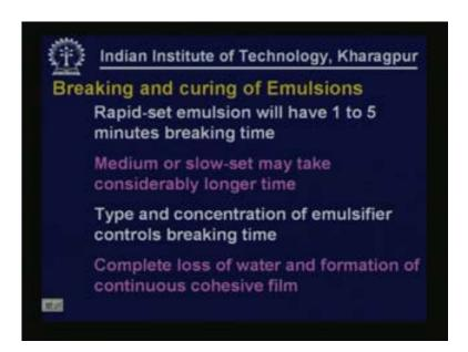
Normally rapid setting emulsions will have about 1 to 5 minutes of breaking time. So, if within 1 to 5 minutes bitumen can coat whatever surface it is suppose to coat then rapid setting emulsion
