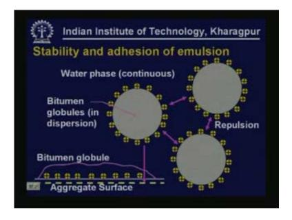
Typically the emulsion can be represented in a pictorial manner in this way. If the entire thing can be considered to be water phase we have bitumen globules although they have shown in a very large and exaggerated manner here and on these globules we have emulsifier adherent on to
