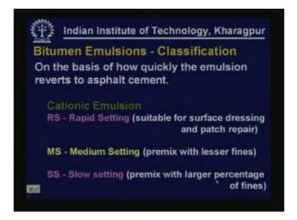
The emulsions can also be classified on the basis of how quickly the emulsion is reversed to asphalt cement. Ultimately asphalt cement ore bitumen is what we want as our binder so the water has to go away. Hence depending on the process that takes place like how quickly the water goes away and the bitumen coats the aggregates the emulsions are classified such as rapid setting, medium setting and slow setting.
