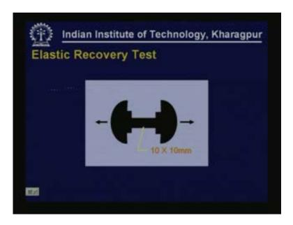
Slightly modified bricket is used. In this case ten by ten millimeters same size is there but it's not at one location but it is over some distance. So this bricket is stretched at same rate of stretching as we do in the case ductility five centimeters per minute.
