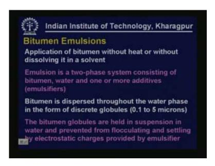
With emulsion it is possible to apply bitumen without heat and without dissolving it in a solvent. That is what we were doing in the case of cutback. In cutback we were reducing the viscosity of the bitumen by dissolving it in a solvent and thereby we are in a position to apply it to the pavement surface. So without doing that and also without applying heat in bitumen emulsions we can use emulsion without the additional need of heat or solvent.
