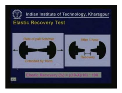
This is extended by 10cm at a rate of 5cm per minute and cut. After one hour we examine that there is some amount of recovery. So these two parts of brickets are bought brought together, its dimension is measured known as x, so elastic recovery is calculated as 10 that's the total
