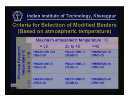
Let us examine the criteria that we have to adopt for selecting appropriate modified binders for different conditions. Usually these are based on atmospheric temperature. On the left hand side we have minimum pavement temperature ranging from -10 to +10 more than 10 and on the upper row we have maximum atmospheric temperature less than 35, 35 to 45 more than 45 and various combinations of modified binders that can be used are listed here.
