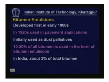
This has been developed first in the early 1900s. In 1920s emulsions were used in pavement applications. That was almost the first known application of emulsion in pavement application and these were initially used as dust palliatives to control dust problems. About 10 to 20% of all bitumen is used in the form of bitumen emulsions that's the world average whereas in India we are using about 3% of the total bitumen that is produced or rather that is used.
