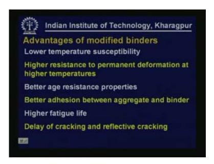
What these modifiers do to the binders? The main advantages of using these modified binders are the temperature susceptibility of modified binders is in general much lower compared to straighten bitumens. That means the properties do not change significantly with temperature variation. These binders have higher resistance to permanent deformation at higher temperatures. In fact this is the main purpose for which usually modified binders are used.
