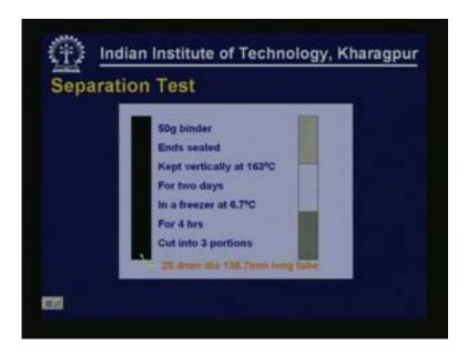
On the left hand side let's consider that to be a vertical tube which is filled with bitumen. About 50g of binder is used, the ends of this tube will be sealed, it is kept vertically at 163 degree centigrade in an oven it is kept like that for two days and after that it is taken out and kept in a freezer at 6.7 degree centigrade for four hours then this bitumen becomes quiet hard and now the tube can be cut into three parts without the bitumen coming out.
