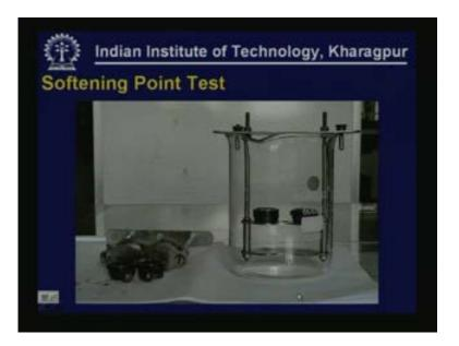
This is a typical arrangement that can be used. Of course I am not showing the complete heating arrangement and other things. We have the frame and we also have the rings and balls are shown on the left hand side.
