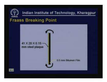
Typically what is done is there is a steel plate on which the bitumen is coated, 0.5mm bituminous film is coated on the steel plate and the temperature of the bitumen is gradually reduced to very low temperatures and then we keep on flexing the bitumen. The temperature at which the bitumen film gets cracked is the Fraass breaking point temperature.
