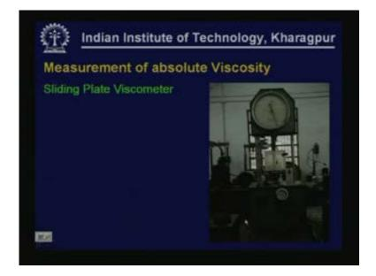
This is a typical set up used for determining the absolute viscosity using a sliding plate viscometer.
