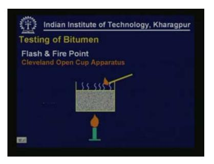
In this the commonly used test method is a Cleveland Open Cup the COC apparatus method. In this method the bitumen is heated gradually as the vapors come, fire is put to that and then if you can observe a flash that is flash point temperature and the temperature at which the vapors start catching fire is the fire point temperature.
