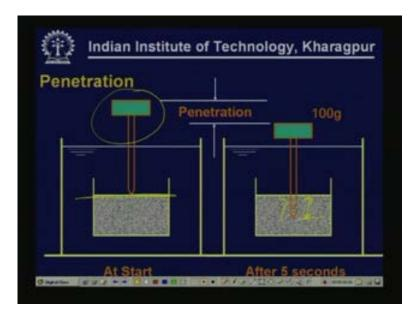
This is the simple schematic arrangement of penetration test. On the left hand side which is at the beginning of the test the needle just touches the surface of the binder and this is the mass including weight of needle (Refer Slide Time: 36:40) and after 5 seconds the needle penetrates into the bitumen, so this is what we are trying to measure and this is the penetration at this temperature.
