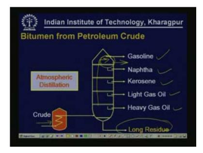
This is a schematic arrangement of the first step of refining of crude which is atmospheric distillation. Here the crude is fed into this and then heated and then fed into this tank so the
