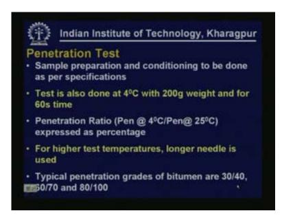
The sample has to be prepared and conditioned in water so that it attains a standard temperature of 25 degree centigrade. There are specifications available for carrying out this test. The test can also be conducted at 4 degree centigrade but with much heavier weight which is 200g and for longer time period which is 60s time. And the penetration ratio which is the penetration at 4 degrees divided by penetration at 25 degree centigrade expressed as percentage is often used to
