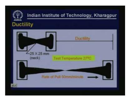
This is the standard briquette that we use having a minimum size of 25/25 at its neck and this is extended at a rate of 50mm per minute. Normally the test is conducted at 27 degree centigrade so the briquette is extended at this rate and when the thread breaks we measure the distance by which it has been extended and that is the ductility of the bitumen.
