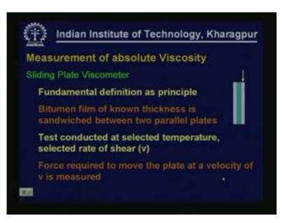
Measurement of absolute viscosity we normally use what is known as the sliding plate viscometer which operates on the basis of the fundamental principle of the definition of absolute viscosity. In this bitumen film of known thickness is sandwiched between two parallel plates. The test is conducted at a selected temperature and at a selected rate of shear that's velocity, and the force required to move the plate at a velocity of v is measured.
