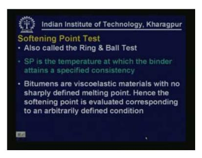
Another very important is that is conducted on bituminous binder is softening point test which is also called as ring and ball test. Softening point is the temperature at which the binder attains a specified consistency. As we know bitumens are visco-elastic materials with no sharply divided melting point. Hence the softening point is evaluated to corresponding to an arbitrarily defined condition. In the next slide let us see what this defined condition is.
