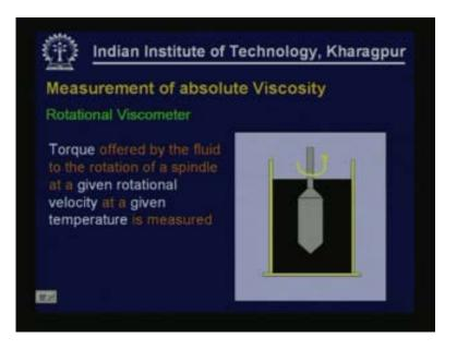
But more commonly used viscometer that is being nowadays used is a rotational viscometer. In this the absolute viscosity is obtained by measuring the torque offered by the fluid to the rotation of a spindle at a given rotational velocity at a given temperature and this has to be measured. Once you measure this torque you can calculate the absolute viscosity of this bitumen.
