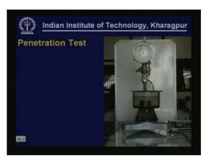
This is a simple apparatus that can be used for conduction penetration test. There is a dial which indicates the penetration.
