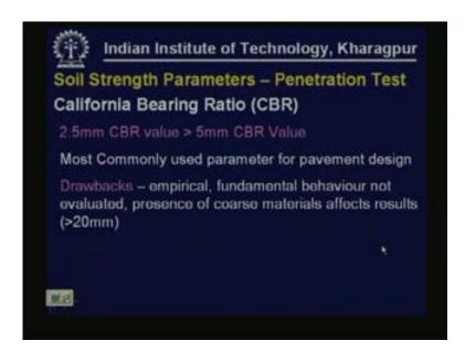
Normally 2.5 mm CBR value is considered that is the ratio obtained corresponding to 2.5 mm penetration is used for design. It is normally more than 5 mm CBR value but if 5 mm value
