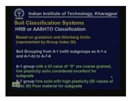
The Highway Research Board or the AASHTO classification is also based on the particle size distribution and the Atterberg limits. There is a parameter called group index GI which is used to
