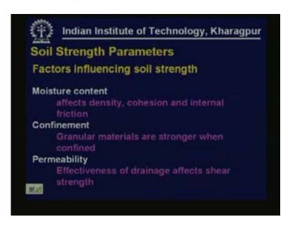
Strength again is influenced by the moisture content which in turn affects the density that is attainable cohesion and internal friction that can be mobilized. In some materials especially granular materials confinement plays a significant role, granular material are usually stronger when they are confined but without confinement they are not so strong. The permeability characteristics of the materials affect the effectiveness of drainage which in turn affects the shear strength of the material.
