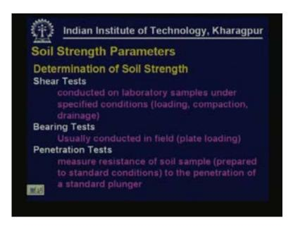
The soil strength parameters or different types of parameters are evaluated. For determining soil strength various types of tests are conducted. These are shear tests normally conducted on
