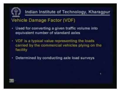
This we have discussed. If you can get information on vehicle damage factor which can be determined by conducting axle load surveys we can convert the commercial vehicles into equivalent number of standard axles.
