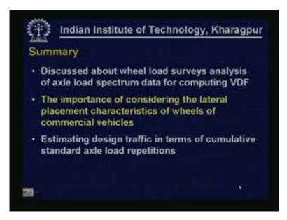
We also discussed about axle load surveys or wheel load surveys that can be conducted and also about the importance of considering lateral placement characteristics of wheel loads of commercial vehicles and we have seen how using all these information equivalent number standard axle loads can be estimated for a design life period.
