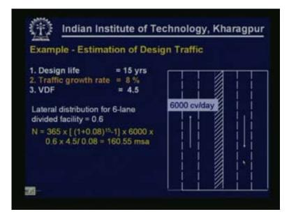
For example, if you take a design life of fifteen years and it traffic growth rate of 8%, VDF of 4.5 and if it is a six lane road divided facility as you have seen in the earlier case we are using a distribution factor of 0.6 so we can work out the number of equivalence standard axle load repetitions as 160.55. In this case we have also used a vehicle damage factor of 4.5.
